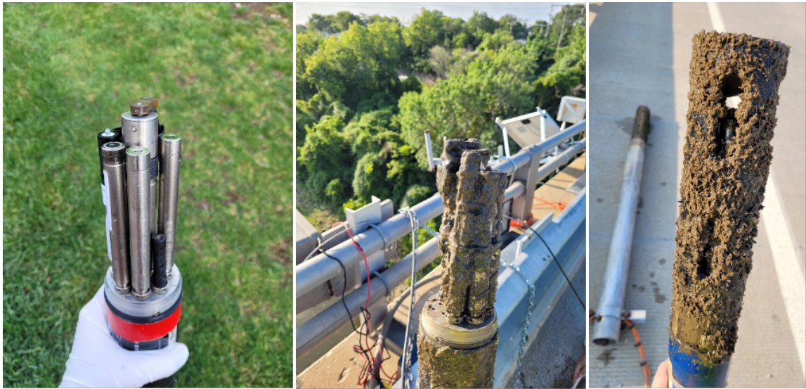
The YSI EXO multi-parameter water-quality monitor measures water temperature, specific conductance, pH, dissolved oxygen, turbidity, and algal fluorescence. Pictured are examples of monitors with heavy biofouling (algal and sediment build up) versus a clean monitor. Photos: Nick Van Nevel.
