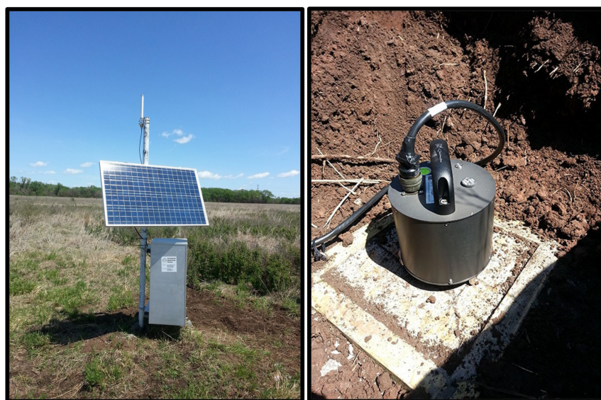
Figure 2. Seismometer installed in Sedgwick County. The seismometer is buried a few feet below the surface (right) and is powered by a solar panel (left). Real-time data are continuously sent to the KGS from every station and can be viewed on the KGS website ( https://www.kgs.ku.edu/Geophysics/Earthquakes/network.html ).
