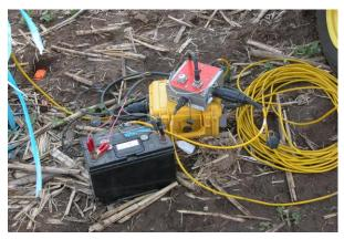
Twenty-four channel Geodes connected to digital line (Ethernet, yellow cables) and then to the controller. Current system includes 480 channels with 100Mbit transmission speeds.
