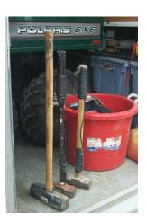
A sledgehammer is a large metal mass, elongated and fitted to a wood or fiber shaft.
