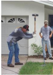
handles and attaching new hammer switches should only be done by experienced KGS staff. A minimum clear area directly in front of the operator of at least 25 ft must be maintained in case operator loses grip on hammer or hammer head breaks free from the handle. Gloves, safety glasses, steel toed boots, and hearing protection are required for operating this source.
