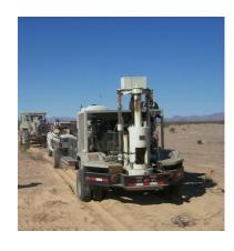
raise and lower the gun chamber to the ground. The gun chamber is hydraulically lowered to the ground with the weight of the truck used to hold the device to the ground. The gun is electrically detonated from the cab of the truck with no moving parts exposed during detonation. The engine and air compressor are enclosed in a protective shroud. The gun generates a thump to the ground surface approximately equivalent to 1/8 of a pound of high explosive buried 3 to 4 ft beneath the ground surface.
