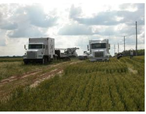
MPC and utility trailer in a field in central Kansas. Seismograph is connected to MPC processing network by Ethernet while seismic data is being recorded using RAWD and towed spread.
