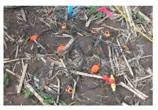
Triple 23 Hz Sensor geophones planted in a 3 ft array.
