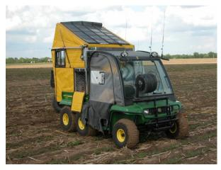
Computer system mounted on a 6-wheel John Deere Gator with rear operator seat is the heart of the 480-channel Geometrics Geode distributed seismograph. Also mounted in this aluminum operator's shell is an IVI Vib controller, time break conditioners, VHF radio, and charging systems powered by four deep-cycle marine batteries that are charged by a roof-mounted solar panel.
