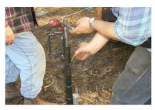
The downhole .50-caliber seismic source consists of a .50-cal. rifle bolted to a 0.6 cm thick steel plate. The rifle itself is a standard .50-cal. breech and bolt, built by Texas Gun and Machine Company, attached to a standard .50-cal. machine gun barrel. Machined
