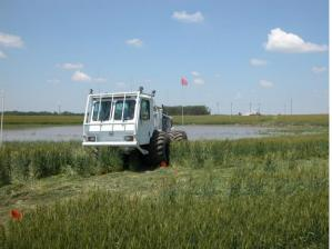
IVI Minivib2 with a sweep range from 10 Hz to 250 Hz and peak force around 13,000 lbs.
