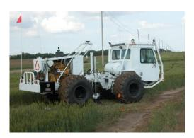
vibrated by a hydraulic servo delivering frequency-varying energy to the plate over a preset time duration. No moving parts are exposed with the maximum movement of the pad relative to the vehicle less than 2 in.
