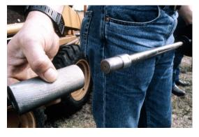
energy. After the source is properly loaded into the borehole a firing rod impacts the primer of the shotgun shell via firing rod that extends through the center of the pipe. Accelerating this firing rod inside the pipe is accomplished with a rubber mallet by impacting the top of the rod. The mallet is instrumented with a contact closure devise that acts as a time zero indicator.
