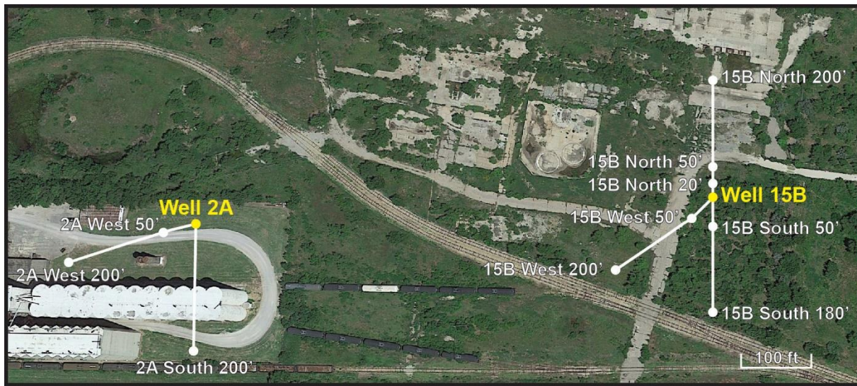
Figure 1. Layout of VSP surveys relative to wells 2A and 15B.
