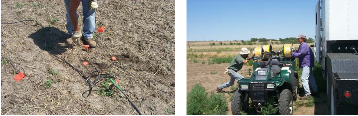
Figure 73. Geophones were planted (left) in a 0.3 m equilateral triangle centered on the DGPS-located station. Weatherproofed reinforced Ethernet cables stored on spools (right) connected the eleven 24-channel Geometrics Geodes to the NZC seismic controller. These cables were deployed using a custom cable handling system.
