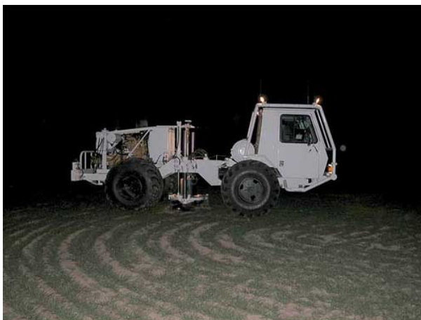
Figure 111. IVI minivib2 working in a field of winter wheat in total darkness. Auxiliary lighting has been installed on this machine providing an enhanced view of the mass and baseplate system as well as the ground around the vibrator cab.
