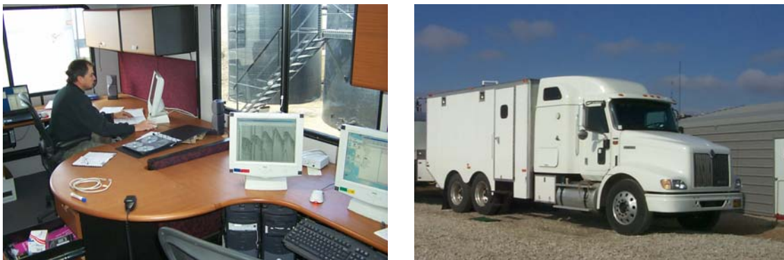
Figure 21. View from front of truck toward computer workstations (left); processing box (right) is climate controlled and mounted on truck frame with ride-controlled air suspension. A 12-kilowatt generator provides both 240-volt and 120-volt power. As data were acquired they were transmitted via Ethernet from the seismograph to the mobile processing center. Once data were transferred, preliminary processing was performed, which included long-term archive, format conversion, pre-correlation processing, correlation, noise editing, vertical stacking, application of geometry, and data inspection.
