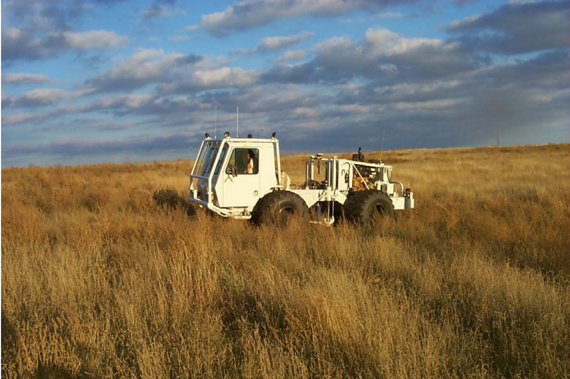
Figure 91. David Thiel operating the IVI minivib2 with GPS tracking and guidance system. A two to four times increase in power was obtained after installation of an Atlas rotary style servo valve in comparison to the factory Moog valve.
