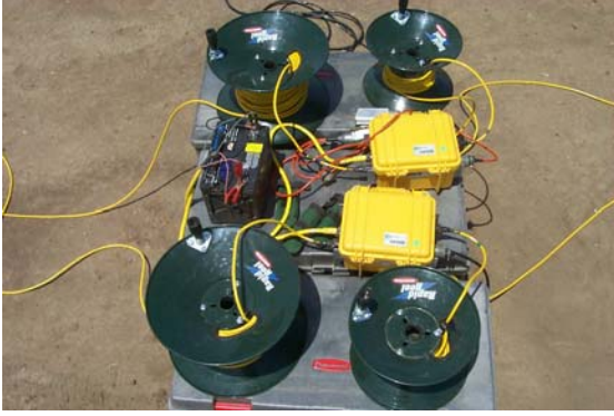
Figure 10. One of five Geode deployments (left) located in the center of each 48-station receiver line. The five Geode groupings were all connected to the Geometrics StrataVisor NZC seismic controller (right). Conducted from this John Deere Gator, seismic operations were all-weather and all-terrain. Here the Gator is configured for warm, dry conditions. Under wet or cold conditions an additional zip-on covering can be added to protect the operator and seismographs.
