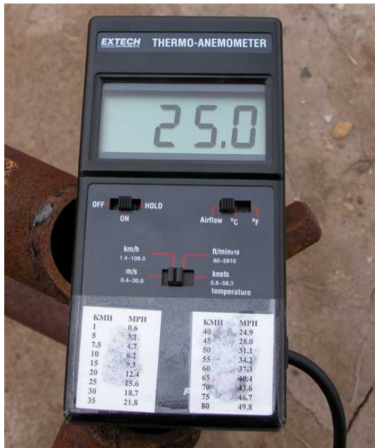
Figure 100. An anemometer to allow accurate measures of wind speed correlated to those previously judged using a windsock and National Weather Service reports. When average wind speeds exceeded 15 m/h (approx. 25 km/h), the survey was halted.
