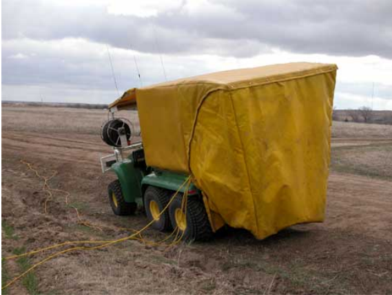
Figure 107. John Deere Gator outfitted with cold weather cover. Propane heater keeps operator's area at room temperature when outside temperatures are well below 0°F.
