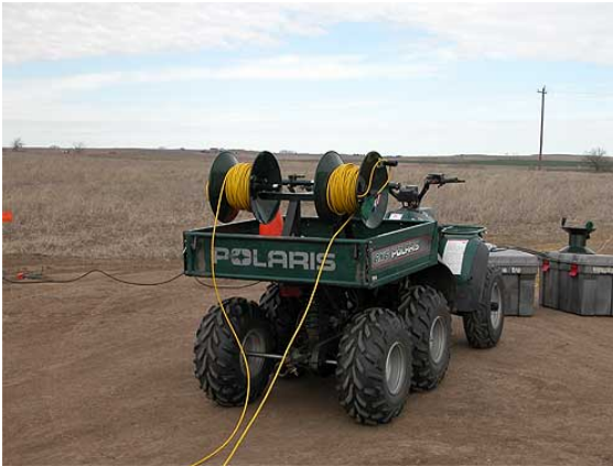
Figure 105. A six-wheel-drive Polaris ATV with two Ethernet cable reels on a four-reel customized bracket.
