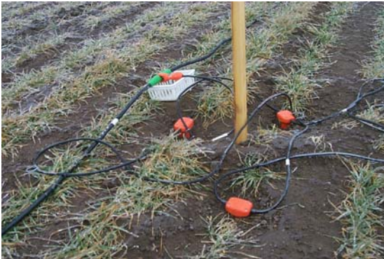
Figure 32. Ten-hertz geophones with tubs to insulate connector.
