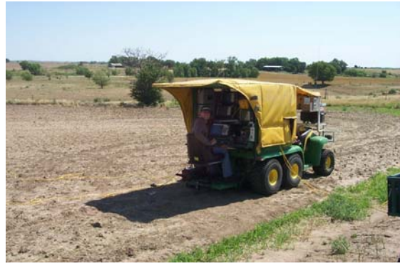
Figure 10. One of five Geode deployments (left) located in the center of each 48-station receiver line. The five Geode groupings were all connected to the Geometrics StrataVisor NZC seismic controller (right). Conducted from this John Deere Gator, seismic operations were all-weather and all-terrain. Here the Gator is configured for warm, dry conditions. Under wet or cold conditions an additional zip-on covering can be added to protect the operator and seismographs.
