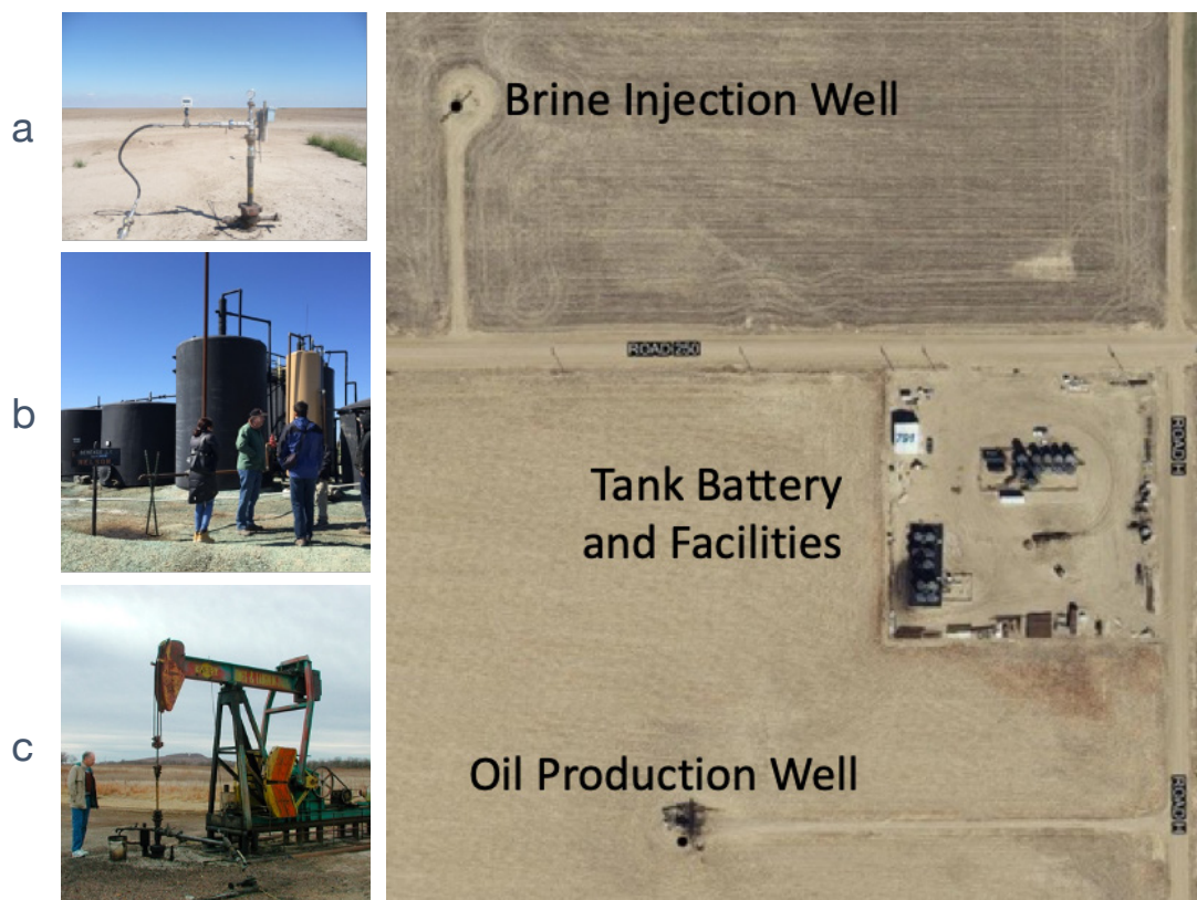
Figure 4. Types of oilfield equipment seen at the Patterson field stop: (a) brine injection well, where co-produced brine is reinjected to maintain reservoir pressure; (b) tank battery and surface facilities, where oil and co-produced fluids such as brine are separated and held—the oil for market and the brine for reinjection; and (c) oil producing well, with its moving pumpjack (also known as a nodding donkey, beam pump, or thirsty bird) that brings oil to the surface.
