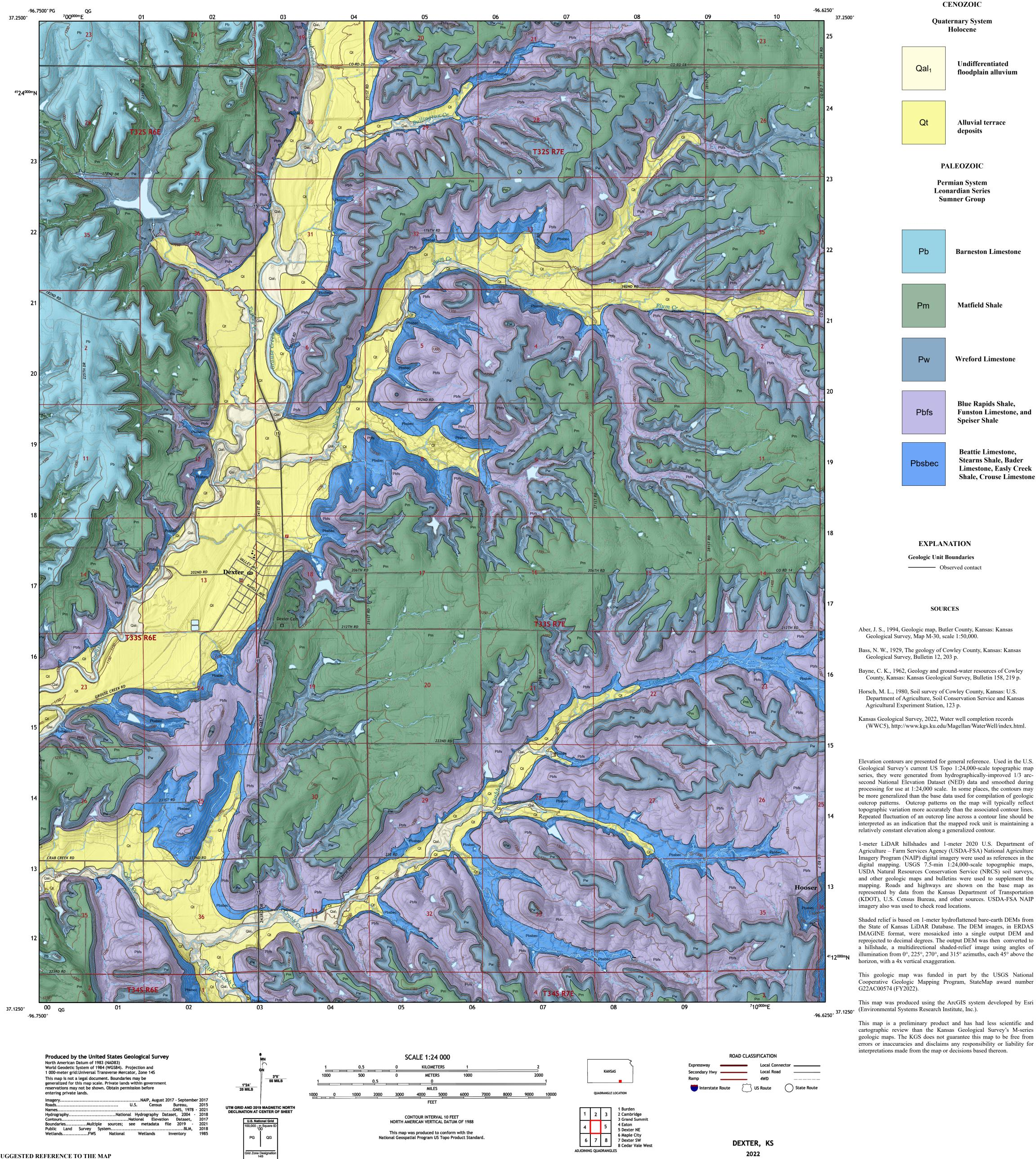
Shaded relief is based on 1-meter hydroflattened bare-earth DEMs from the State of Kansas LiDAR Database. The DEM images, in ERDAS IMAGINE format, were mosaicked into a single output DEM and reprojected to decimal degrees. The output DEM was then converted to a hillshade, a multidirectional shaded-relief image using angles of illumination from 0°, 225°, 270°, and 315° azimuths, each 45° above the
