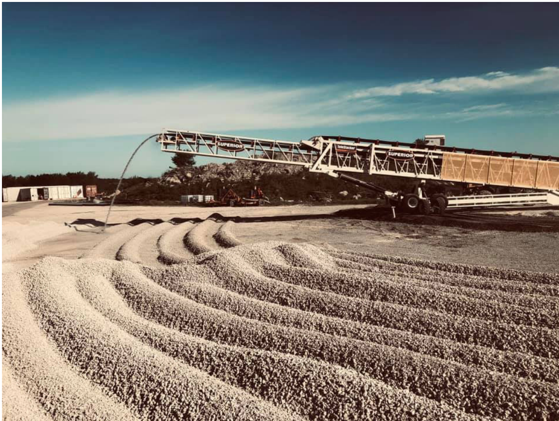
Figure 5. Rock segregation, or variation in size within aggregate materials, lowers the quality of the aggregate. Machines called stackers, like the one pictured here, keep rock segregation to a minimum. (Photo courtesy of Midwest Minerals.)
