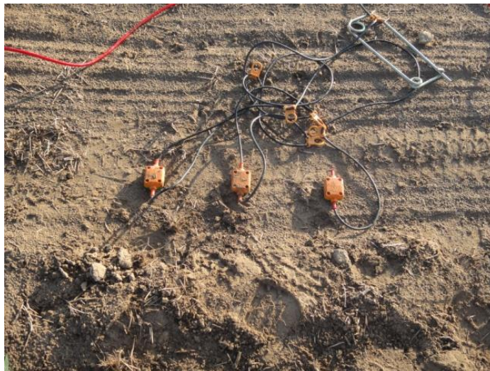
Figure 9. Three L28A 30 Hz Sercel geophones planted in a 3 ft array.
