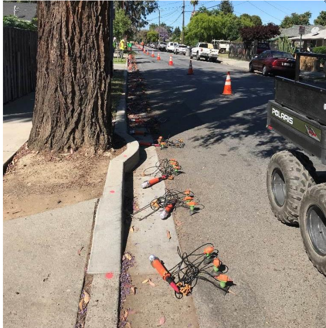
Figure 8. NRU nodes (orange baton shaped object) connected to 3 28 Hz geophones with rock plates.
