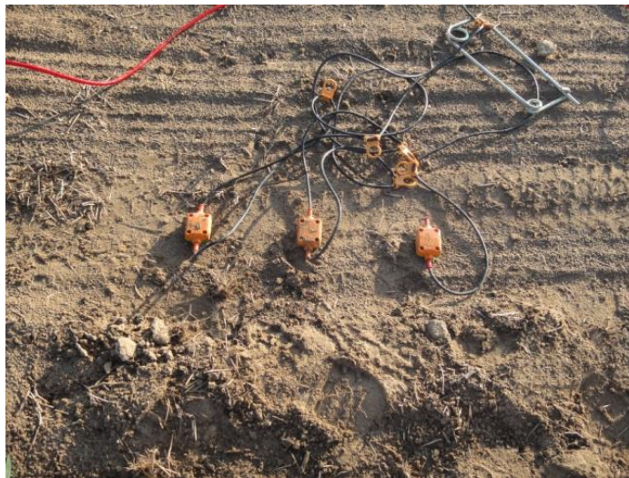
Figure 9. Three L28A 30 Hz Sercel geophones planted in a 3 ft array.
