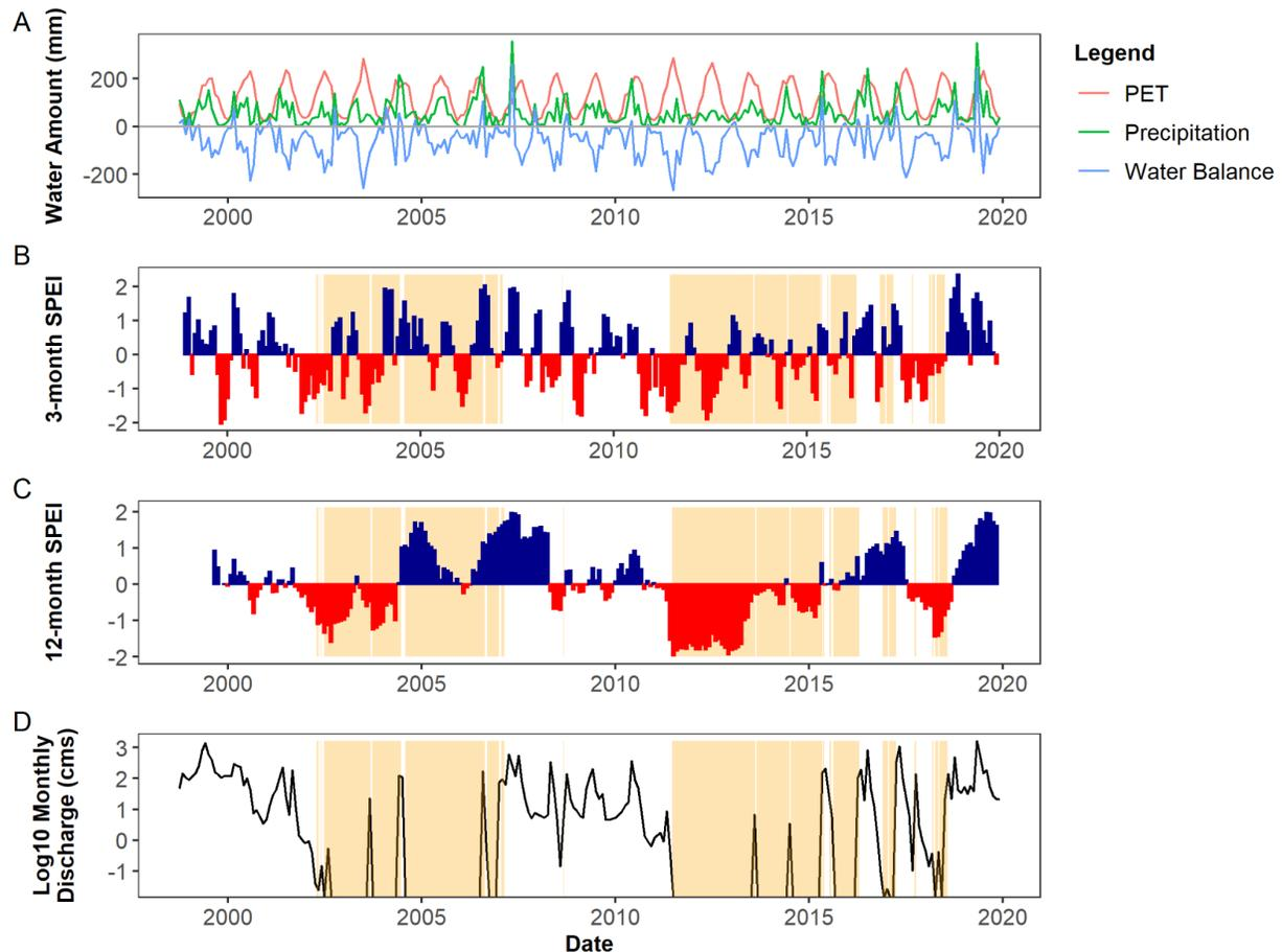
**Figure 10. (a) Meteorological input data at monthly resolution (precipitation, potential evapotranspiration [PET], water balance), where water balance is defined as (precipitation - PET); (b) 3-month SPEI; (c) 12-month SPEI; and (d) mean monthly discharge. For all panels, the dry periods are shaded with an orange background.**
