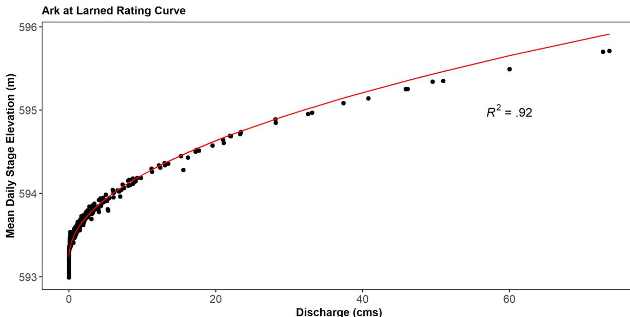
**Figure 12. Rating curve used to back-fill historical stage data based on discharge.**
