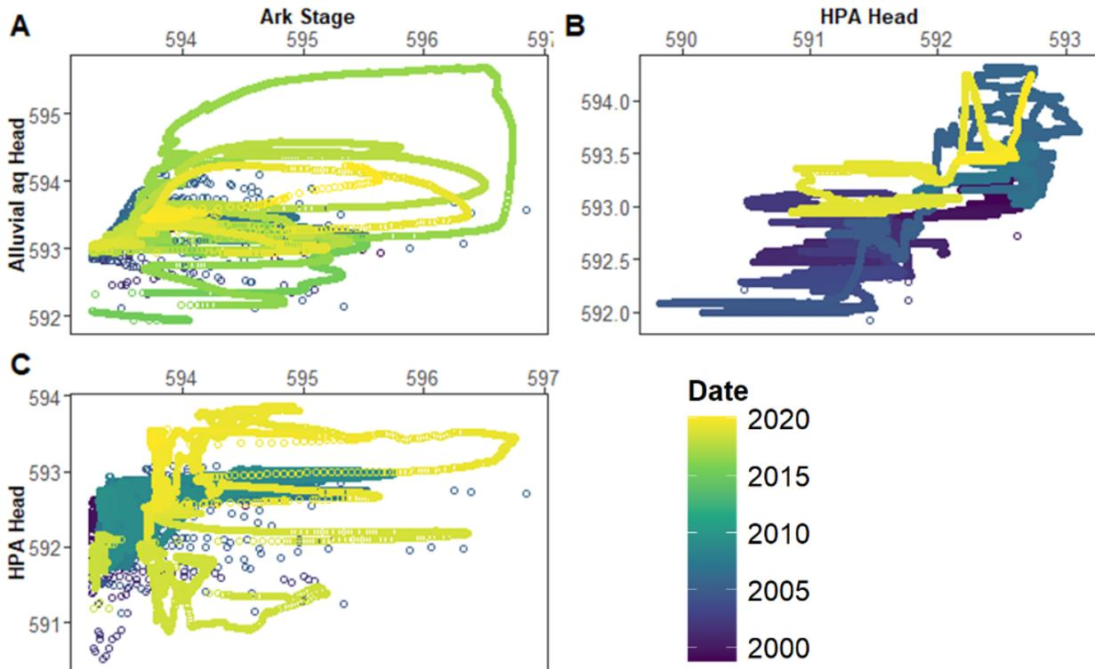
**Figure 14. Plots of (a) river stage vs. alluvial aquifer head; (b) alluvial aquifer head vs. HPA head; and (c) HPA head vs. river stage. River stage values that are equal to the riverbed elevation (i.e., no flow) were removed before plotting.**
