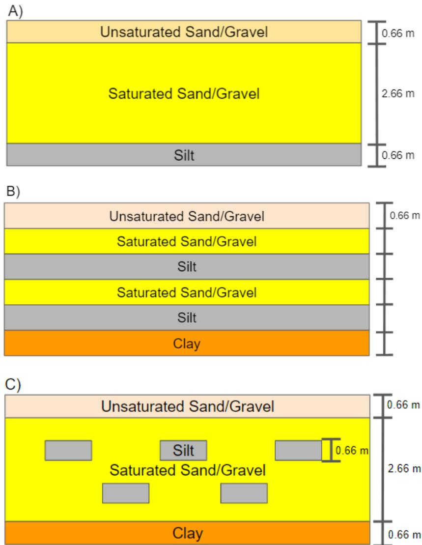
**Figure 17. Three conceptual models that were simulated using forward models. All models are 4 meters thick and 31 meters long: (a) simplest model, (b) vertical heterogeneous model, and (c) vertically and laterally heterogeneous model.**
