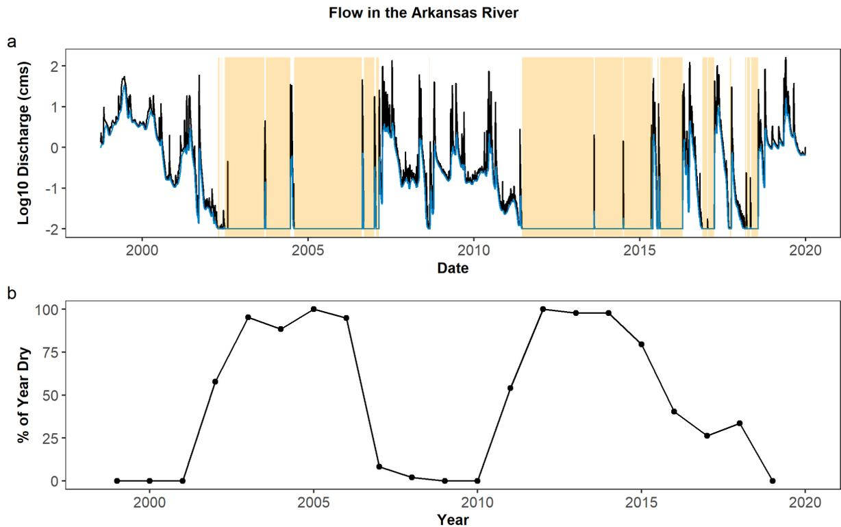
**Figure 2. (a) Logarithmic hydrograph of the Arkansas River at Larned (1998–2019), with zero flow readings plotted as  $10^{-2}$  cms. Streamflow is plotted as a black line and baseflow is plotted in blue. The highlighted sections show dry periods. (b) Annual percentage of the calendar year with zero flow.**
