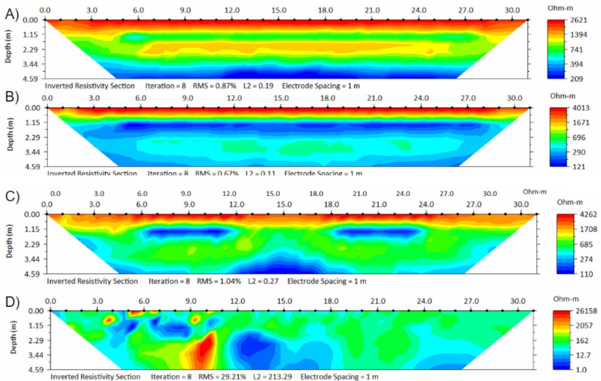
**Figure 18. Forward model inversions using (a) simplest model (fig. 17a), (b) vertical heterogeneous model (fig. 17b), (c) vertically and laterally heterogeneous model (fig. 17c), and (d) inverted data from the Arkansas River sandbar ERT transect for comparison. Note that colorbar limits vary among plots.**
