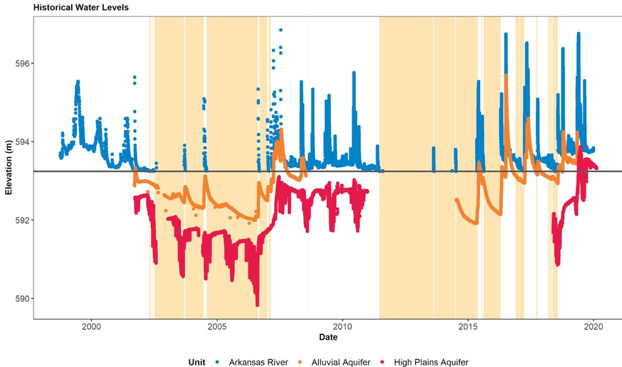
**Figure 13. Time series plot of river elevation, alluvial aquifer head, and High Plains aquifer head. The grey line signifies the elevation of the riverbed.**
