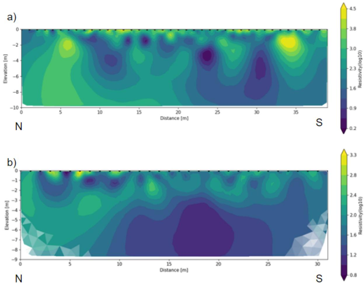
**Figure 16. (a) Inverted ERT profile of the western bank of the Arkansas River, root mean squared (RMS) error = 1.06%, and (b) inverted ERT profile of the sandbar, RMS = 1.13%. N and S indicate north and south ends of transect, respectively. Profile locations are shown in fig. 1.**
