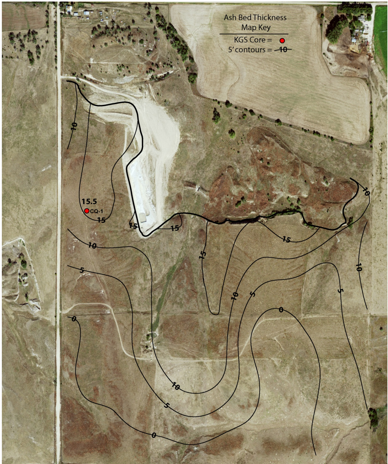
Figure 6. Subsurface isopach map with 5-foot-contour intervals estimating ash bed thicknesses, generally west and south of the quarry face.
