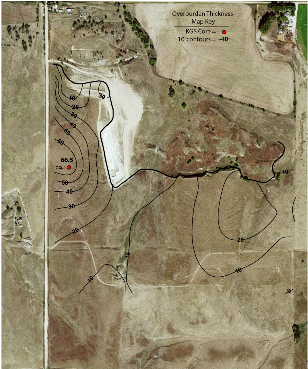
Figure 4. Subsurface isopach map with 10-foot-contour intervals estimating thicknesses of overburden above the ash bed, generally west and south of the quarry face.
