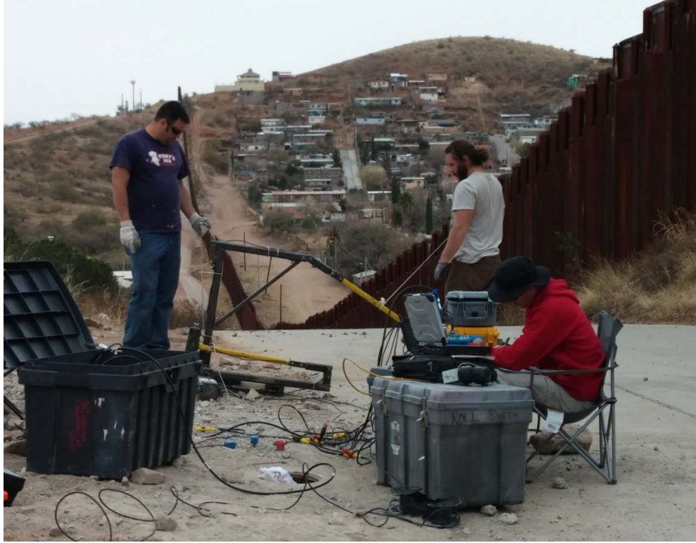
Figure 7: Downhole seismic acquisition at Nog-C_N3 (DTRA N2).
