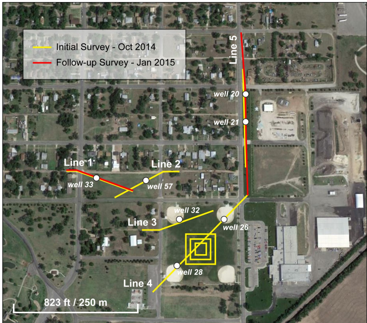
Figure 3. Aerial photo with GPS locations of seismic lines from the initial survey in October 2014 (yellow lines) and follow-up survey in January 2015 (red lines) and locations of wells (white circles) in the study area.
