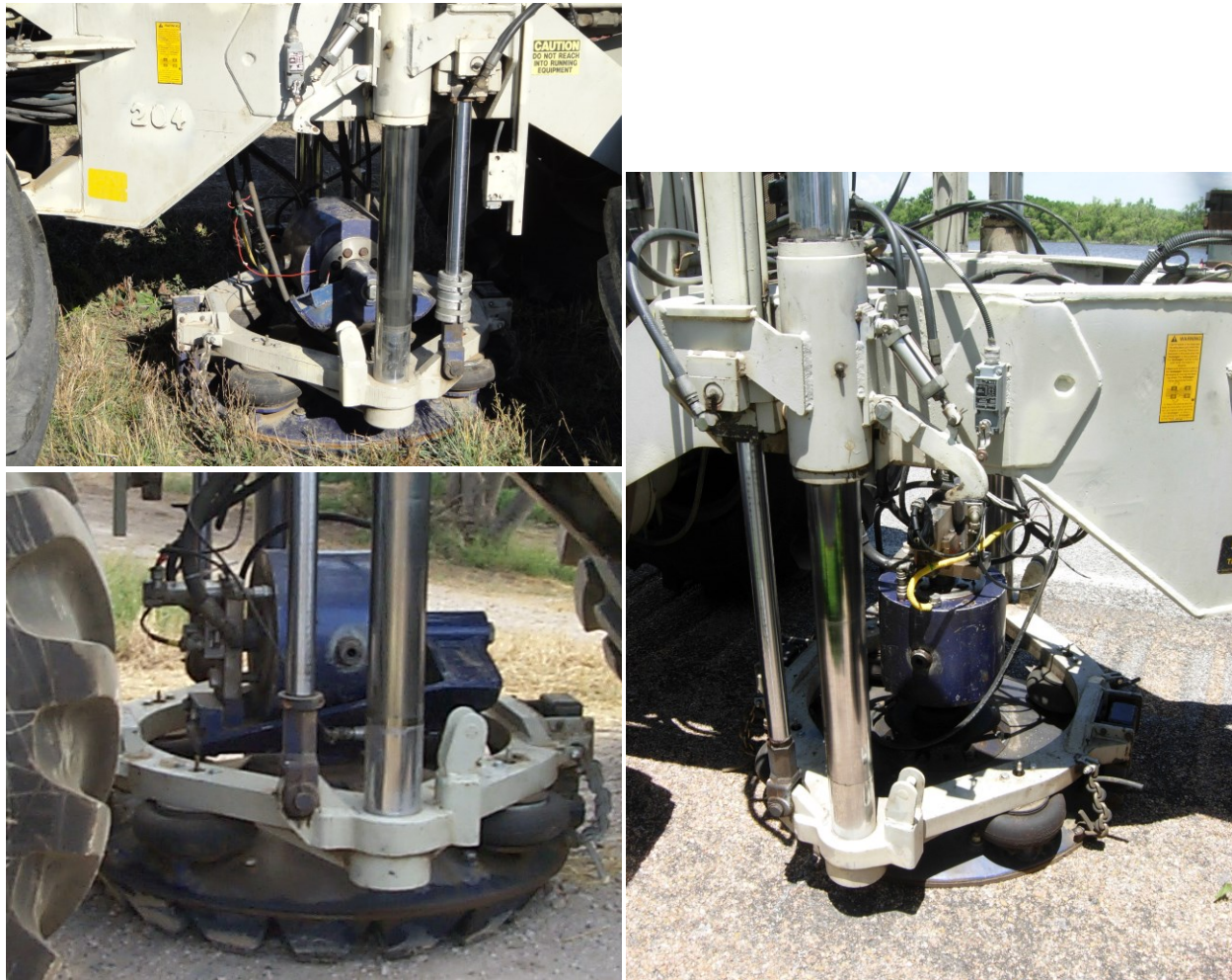
Figure 15: Picture of the IVI Minivib system used at YPG with three different orientations of the hydraulic mass: top left) S_H -; bottom left) S_V -; right) P-wave. Note the waffle plate used for shear generation in the lower left image and that the survey line is parallel to the long axis of the Minivib.
