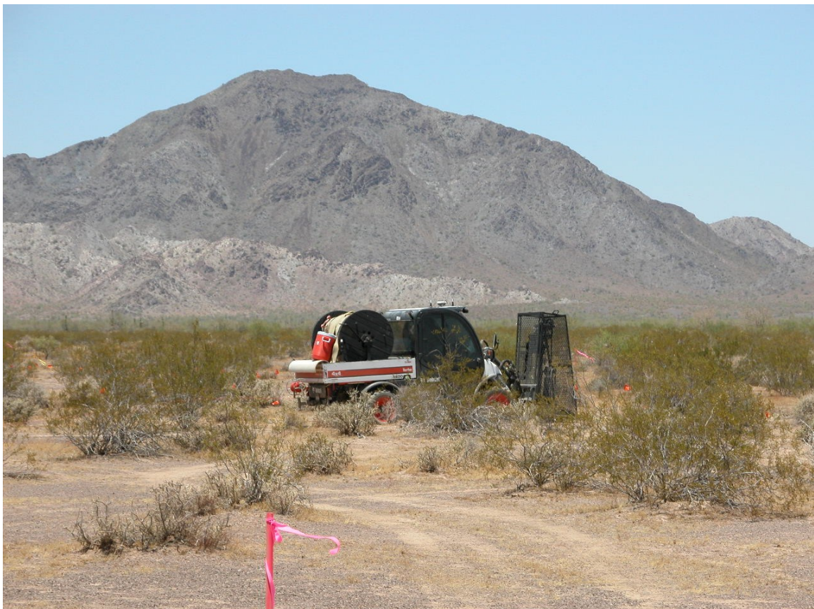
Figure 13: Photo of the weight drop used for P-wave refraction and MASW processing with the Trigo Peaks in the background.
