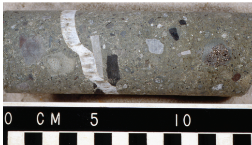
FIGURE 19—Baldwin Creek kimberlite at 256 ft. Many xenoliths and a gypsum-filled fracture.
