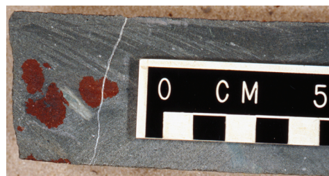
FIGURE 18—Antioch kimberlite at 38 ft 9 inches. Red, iron oxide patches.
