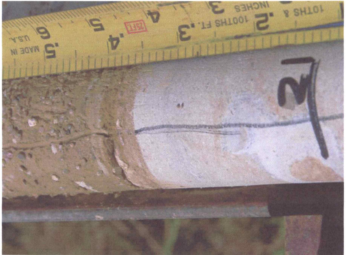
Figure 16- Core showing the contact of the chert bed in Threemile limestone with the underlying unit.
