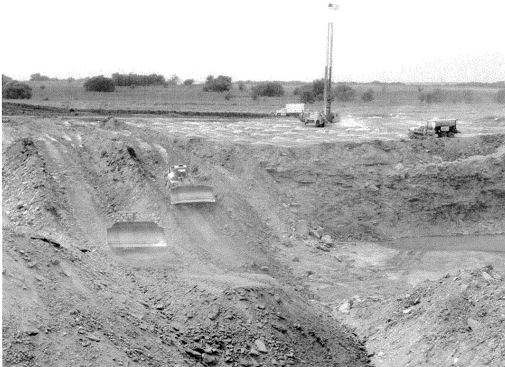
Caterpillar track-type tractors move overburden across pit. Drilling rig prepares holes to blast the overburden.
