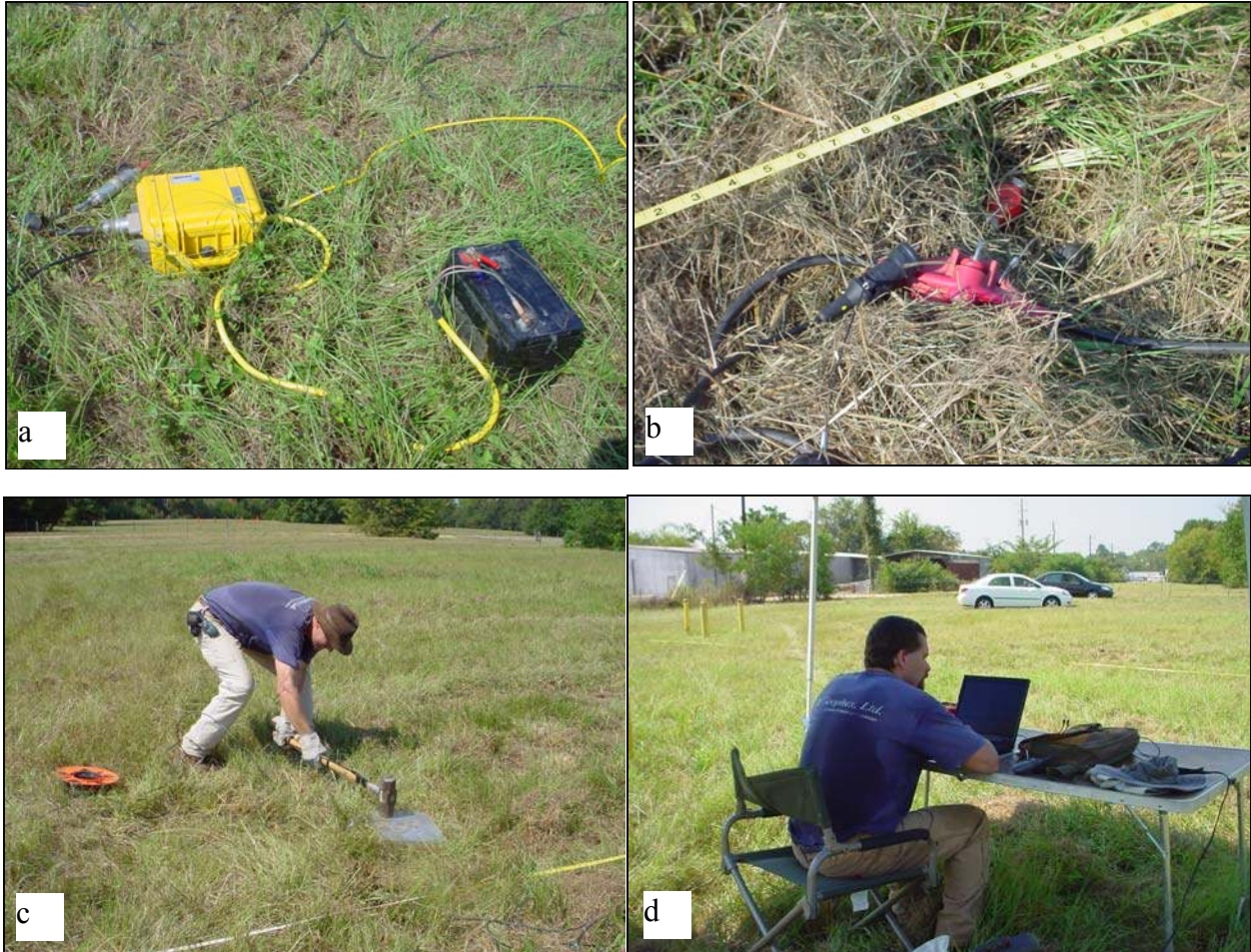
Figure 3. a) One of four Geodes used in data acquisition. b) A 4.5-Hz vertical component geophone. c) A 12-lb hammer vertically impacts a 1 ft by 1 ft metal plate as a seismic source. Karlin Yudichak of Geophex Ltd. was swinging the hammer. d) A notebook was used to record data. Brad Carr of Geophex Ltd. was assessing data.
