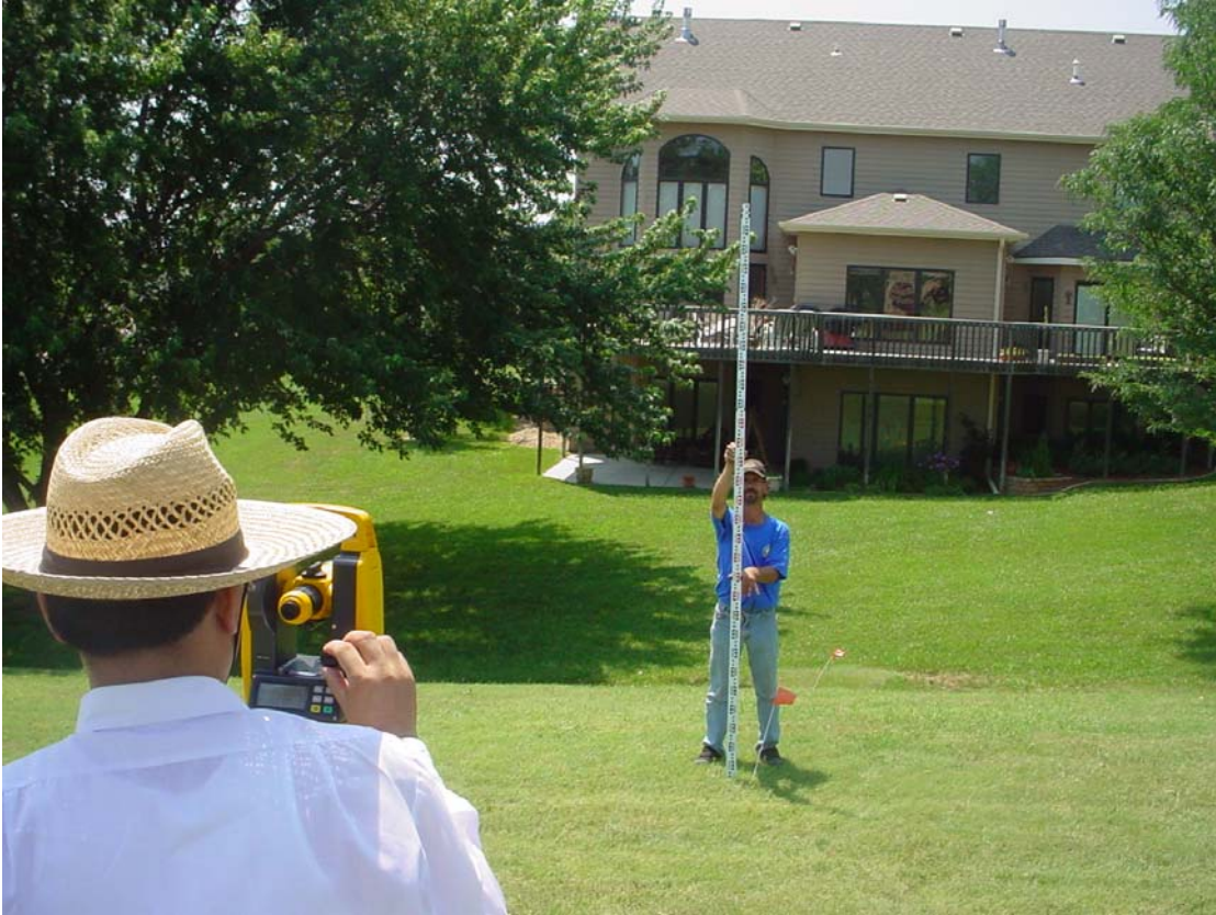
Figure 2. A CST/Berger electronic digital theodolite was used in defining grids, lines, and elevations along line 1.
