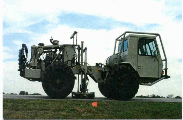
Figure 7. IVI minivib with Atlas rotary valve. Approximately 800 ft-lbs of force can be applied at 100 Hz, while around 2000 ft-lbs are possible in some conditions at 250 Hz.
