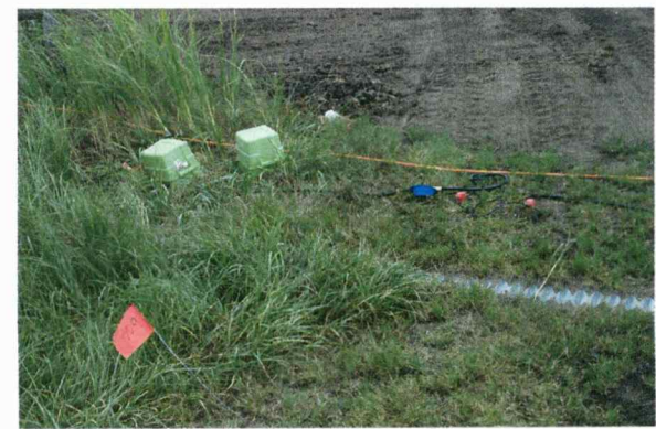
Fig A12. Cable, phones, and support tubs along line 2 on Victory Road.
