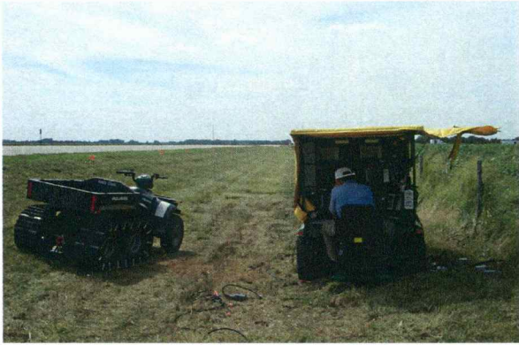
Fig A1. Seismograph mounted in John Deere Gator along seismic line 1 with tracked 6-wheel-drive Polaris cable/phone vehicle.
