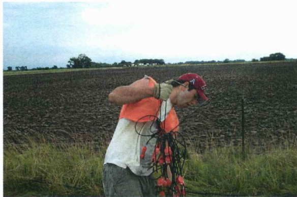
Fig A9. Geophones collected on a metal hasp designed to carry as many as 12 strings.
