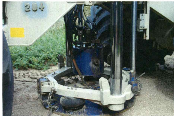
Figure 8. 300 lb mass and 300 lb baseplate with new prototype Atlas rotary valve.
