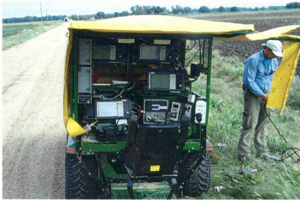
Figure 6. 240 channel Geometrics StrataView with support electronics (line checker, IVI source synchronizer, time break conditioner, etc.).
