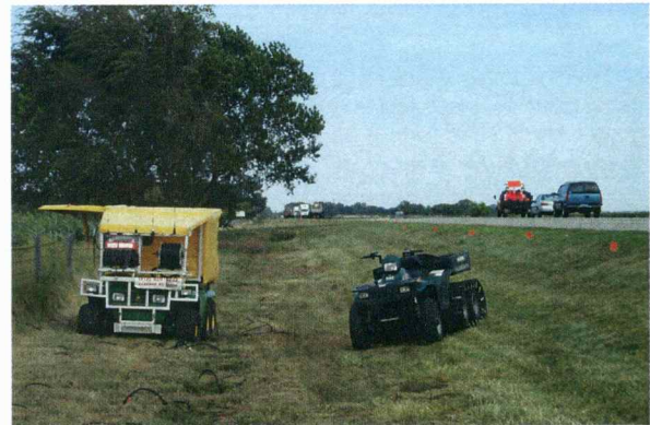
Fig A4. Seismograph vehicle with cables and phones in ditch and KDOT pilot car in the background.
