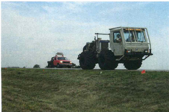
Fig A5. Vibrator along westbound shoulder of U.S. 50.
