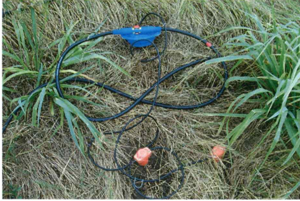
Figure 4. Two Mark Products L28E 40 Hz geophones separated by about 1 ft to form a 2 ft effective array.
