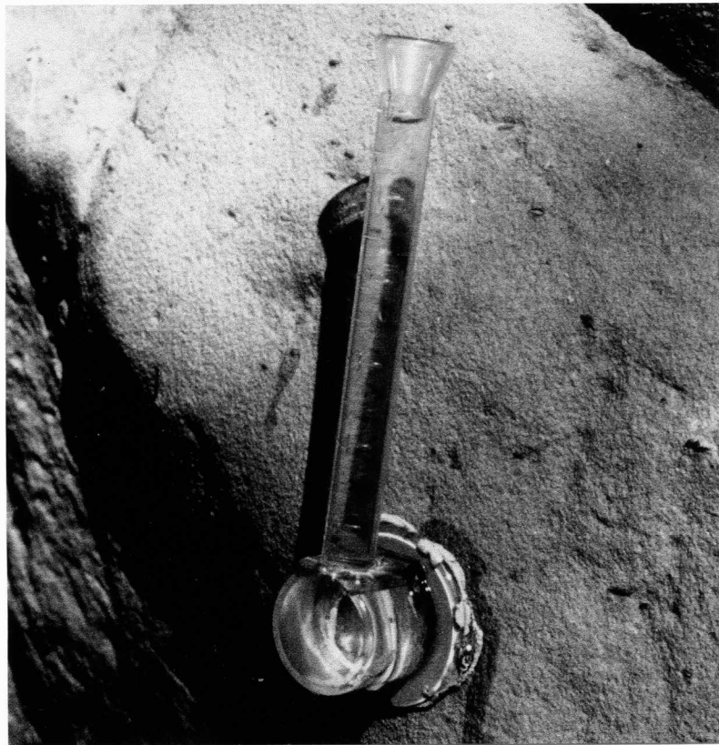
Figure 2. Capillary Tube for Measuring in situ capillary absorption.
