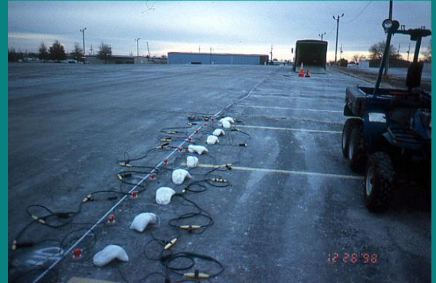
Geophones with baseplates and baseplates with sandbags
