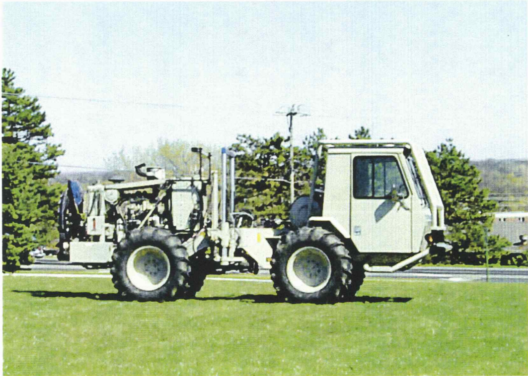
Figure 14. Vibrator truck used as a seismic source.
