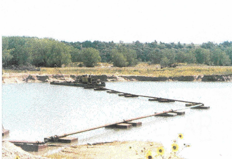
Figure 7. Floodplain dredge. (Midwest Concrete Materials, Inc., Manhattan, KS)
