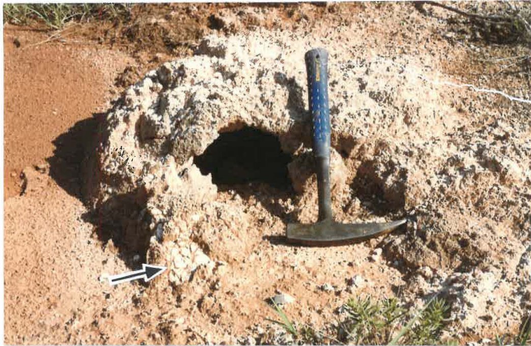
Figure 33: Hollow mound in Blaine Formation gypsum caused by dissolution; note large recrystallized gypsum crystals at base of mound (arrow); hammer for scale is 32.5 cm long; Radio tower hill outcrop, near gate 4, Maria Ranch, Barber County, Kansas; SW1/4, NE1/4, Sec. 29, T32S, R12W.
