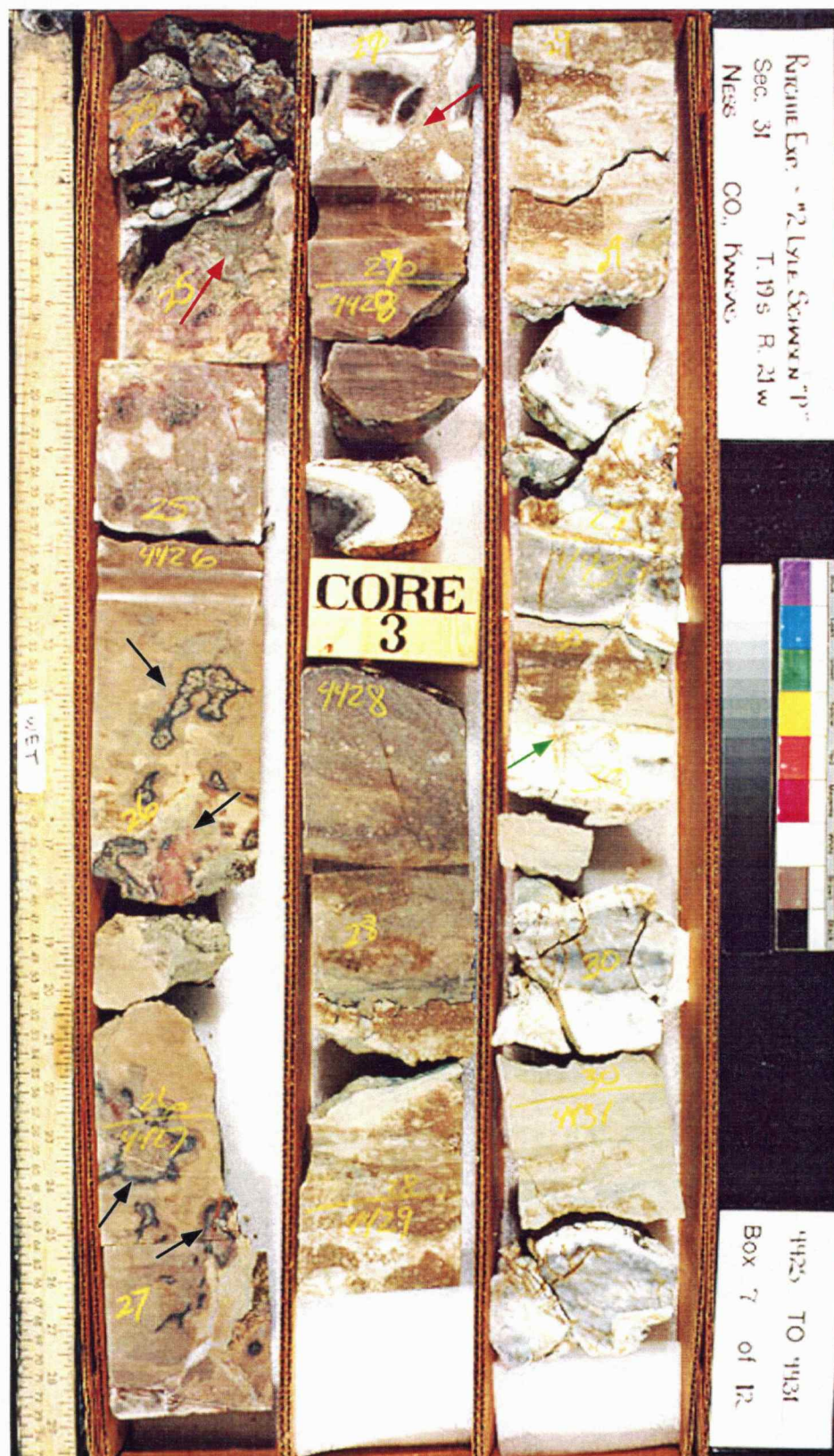
Figure S.4A: Core photo of #2 Lyle Schaben "P" (4425' to 4431'). Black arrows point to iron-stained mottled areas. Petrographic examination indicates some of these altered areas are characterized by a central area filled with coarse calcite cement surrounded by a halo rich in iron and fenestral pores in dolomitic and replacive poikilotopic calcite matrix, which may indicate these are associated with land plant roots (see Figure 10c). The red arrows point to fracturing and brecciation likely associated with the 4424' surface subaerial exposure event. These fractures cut across original dolomite facies, poikilotopic cement replaced facies coarse calcite cement and chert replaced facies (see Figures 10B, D, E, F for petrographic characteristics of these fractured and brecciated areas). Note that the fractured area indicated by the red arrow near the top of the core (~4425.5') was in turn crosscut by a later fracture filled with abundant green clay, possibly associated with the post-Mississippian subaerial exposure event. The green arrow near 4430' points to a fracture in chert that is filled with dolomite matrix from immediately overlying facies. This indicates early chert replacement and fracturing.
