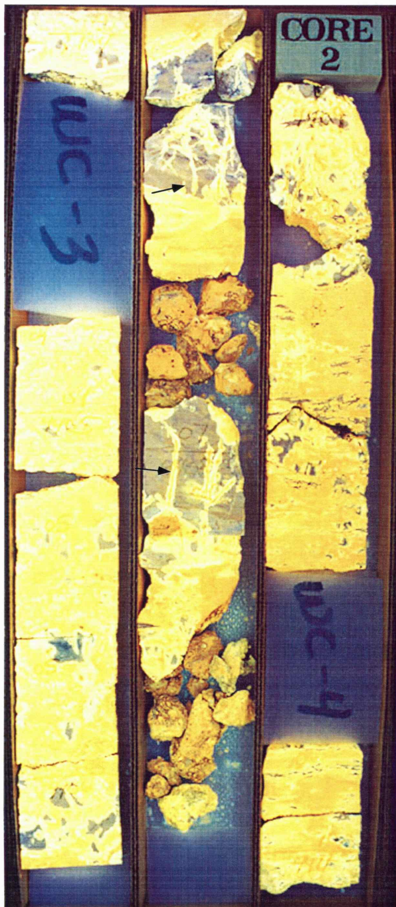
Figure S.2B: Core photo of #2 Lyle Schaben "P" (4403' to 4411'). Same interval as Figure S.2A but taken under UV light. Note that the sponge spicule-rich facies contains abundant oil stains (bright areas) whereas the chert areas are relative tight (dark areas). This photo nicely shows oil stained fractures that cut across some of the chert areas (black arrows).
