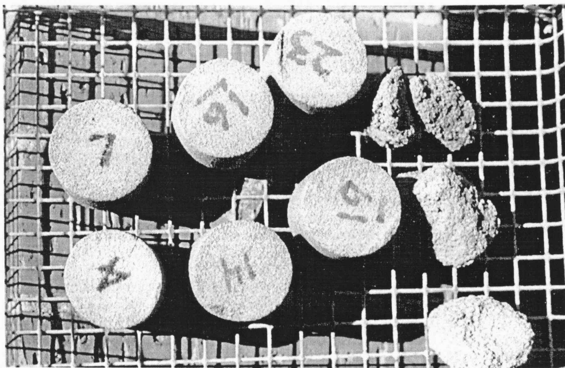
Figure 2. Cores of the Hell Creek Sandstone, Pompeys Pillar, Montana, after 75 freeze-thaw cycles. All of the treated cores appear fresh and unaffected while the two untreated cores on the right have undergone nearly complete destruction.
