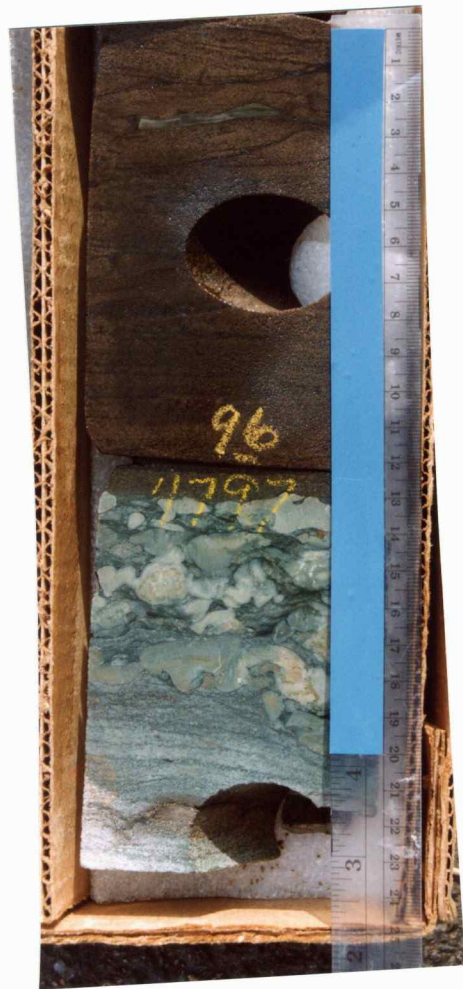
Fig. 61 Carbonate lithoclasts at top of facies D in Scott #4-4 core. Scale bar = 20 cm.
