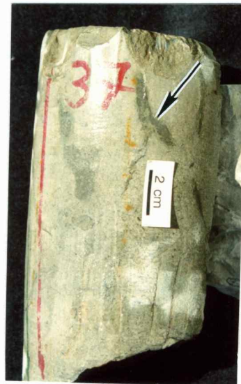
Fig. 21 Green to gray slightly silty micrite filling root molds in facies IP at top sequence j. Scale bar = 2 cm.
