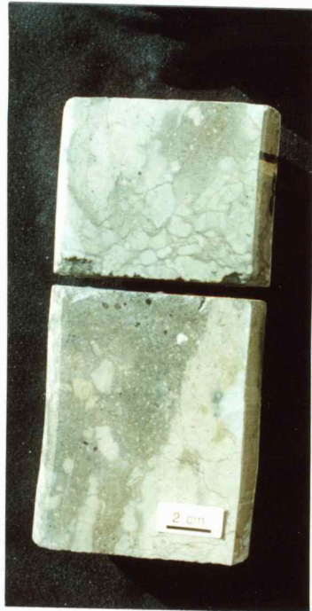
Fig. 31 Photo displays karst fill within sequence k carbonates @ 5289' in the #1 Harris. Scale bar = 2 cm.
