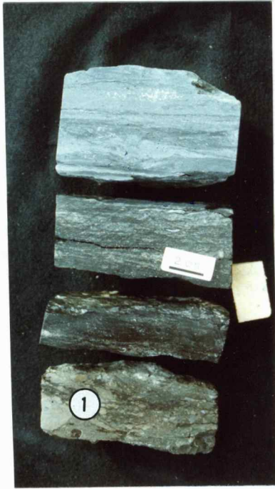
Fig. 12 Facies LP-SH at base of sequence f (4901-4902). Photo shows basal transgressive lag with lithoclasts (1) grading vertically into dark-gray shale and carbonate mudstone to wackestone. Scale bar = 2 cm.
