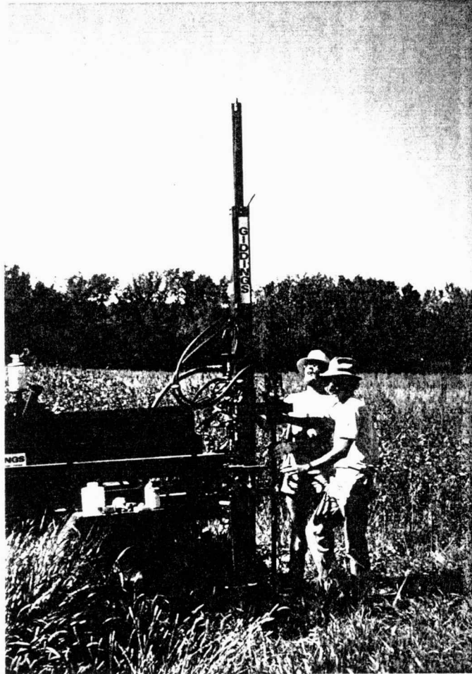
Plate 4:1 Trailer-mounted drill rig (Giddings) used to collect cores from valley and valley side fills.
