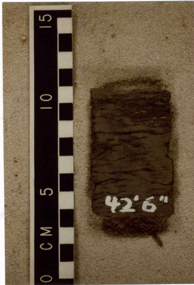
Figure 33: Facies GSH (Grey shale). Paper-thin laminations are characteristic of this Haberer core piece (sec 14 T12S R15W). Footage below KB.
