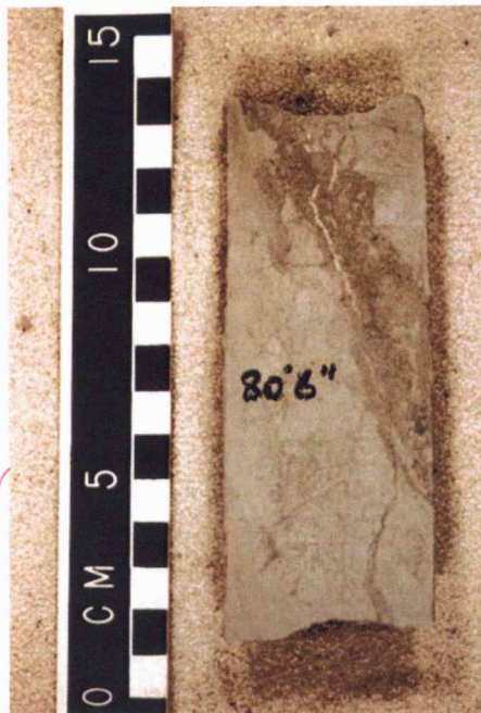
FIGURE 3.15—Mottled sandstone (Facies MTSS). In this core piece, the sandstone is mottled and brecciated from compaction and dewatering. The core piece is from the Haberer test well in sec. 14, T. 12 S., R. 15 W. Footage marked on the core piece is the depth below the KB.
