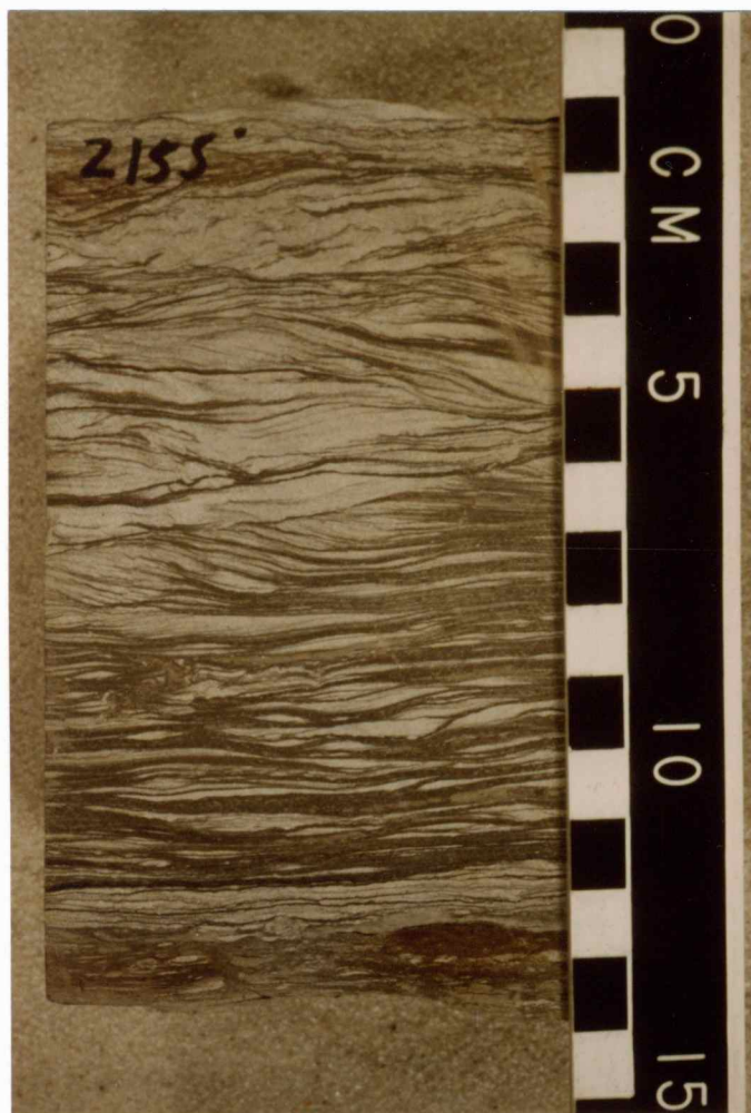
Figure 25: Facies CSS/SH (Carbonaceous interlaminated sandstone and shale). This piece of the Beaumeister core (sec 31 T2S R39W) exhibits lenticular and flaser bedding, and climbing ripples. Amount of carbonaceous material in fine laminations varies in this facies. Footage below KB.
