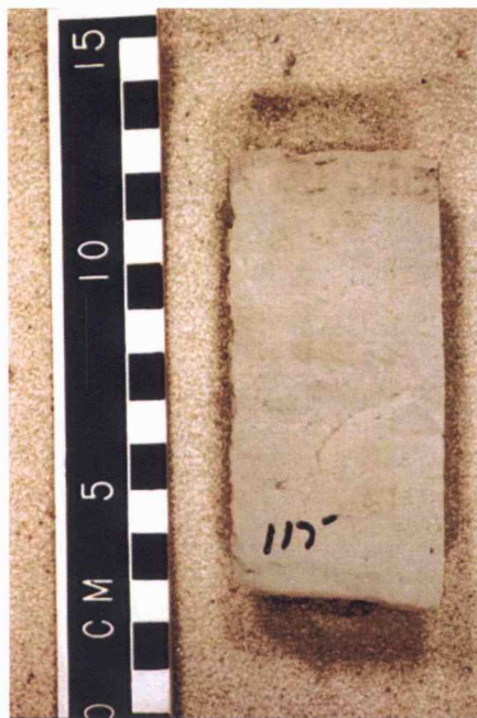
FIGURE 3.14—Siltstone (Facies ST). Note the massive texture that can be seen in this piece of the core from the Haberer test well in sec. 14, T. 12 S., R. 15 W. Footage marked on the core piece is the depth below the KB.
