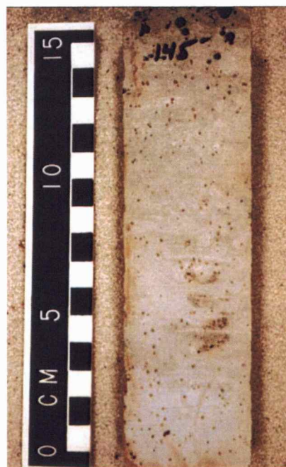
FIGURE 3.16—Mottled sandstone (Facies MTSS). Sideritic spherulites and faint laminations are visible in this piece of core from the Haberer test well in sec. 14, T. 12 S., R. 15 W. Footage marked on the core piece is the depth below the KB.
