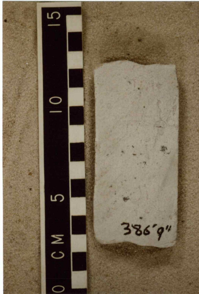
Figure 16: Facies PSS/SH (Pyritic interlaminated sandstone and shale). Few shale laminations are present in this part of the Haberer core (sec 14 T12S R15W). Footage below KB.
