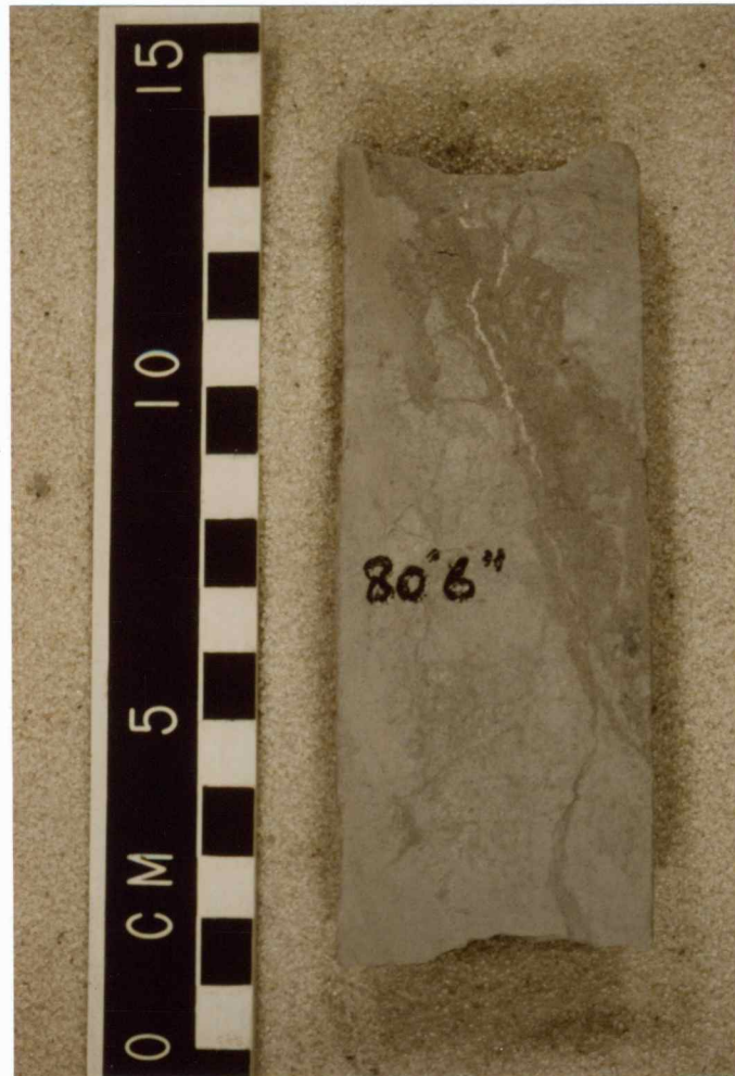
Figure 22: Facies MTSS (Mottled sandstone). This Haberer core piece (sec 14 T12S R15W) is mottled and brecciated from compaction and dewatering. Footage below KB.
