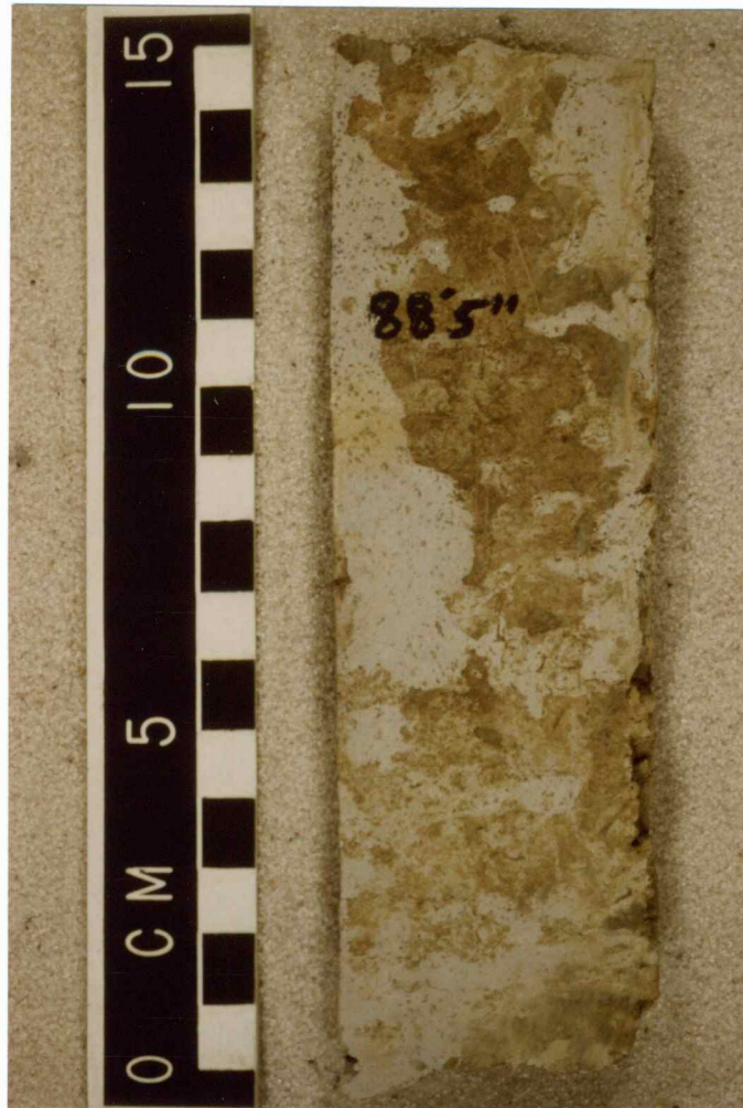
Figure 18: Facies VGMS (Variegated mudstone). Yellow and brown variegations and sideritic spherulites are present in this Haberer core piece (sec 14 T12S R15W). Footage below KB.
