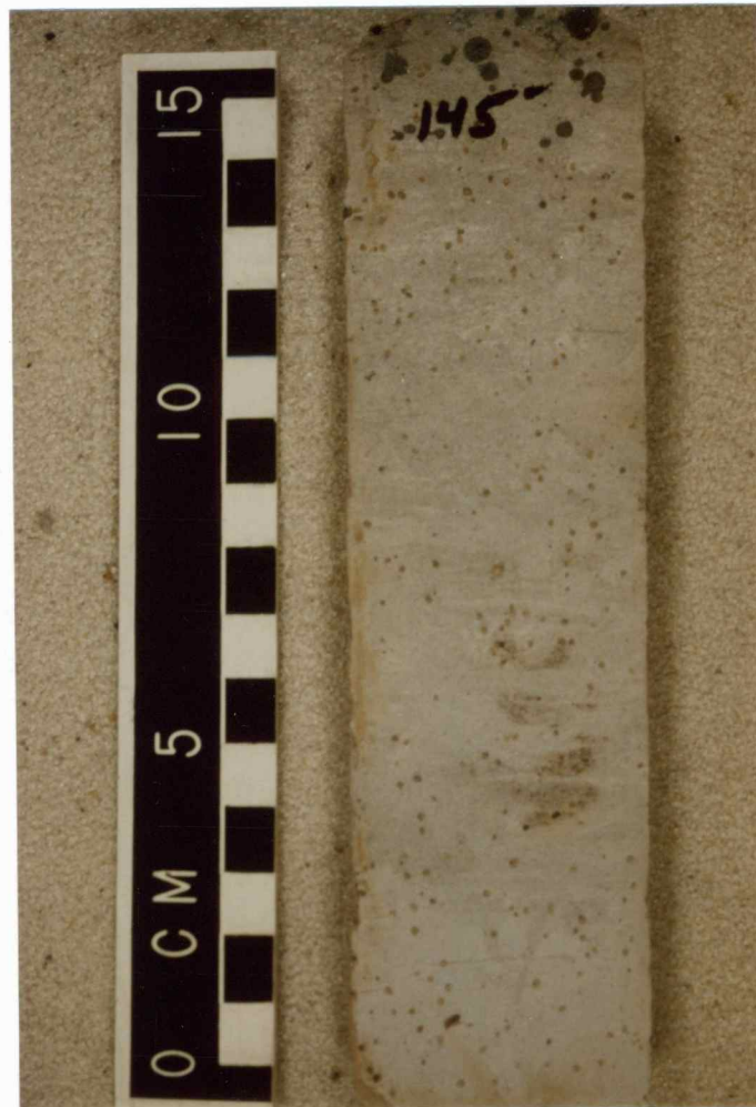
Figure 23: Facies MTSS (Mottled sandstone). Sideritic spherulites and faint laminations are visible in this piece of the Haberer core (sec 14 T12S R15W). Footage below KB.
