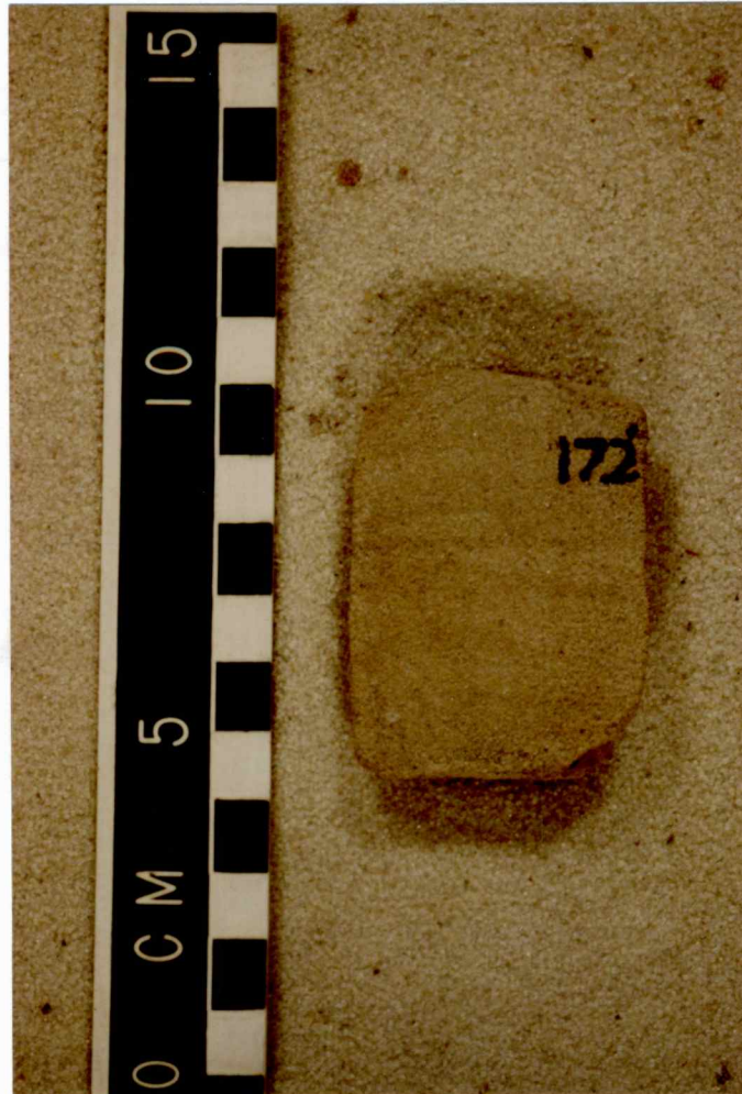
Figure 13: Facies STXSS (Small-scale trough cross-stratified sandstone). This piece is from the Haberer core (sec 14 T12S R15W). Footage below KB.
