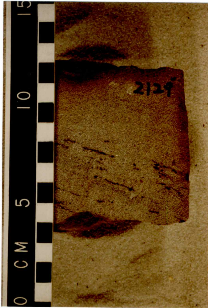
Figure 12: Facies STXSS (Small-scale trough cross-stratified sandstone). Cross stratification seen in this core piece from the Beaumeister core (sec 31 T2S R39W) has flattened wood pieces between laminae. Footage below KB.
