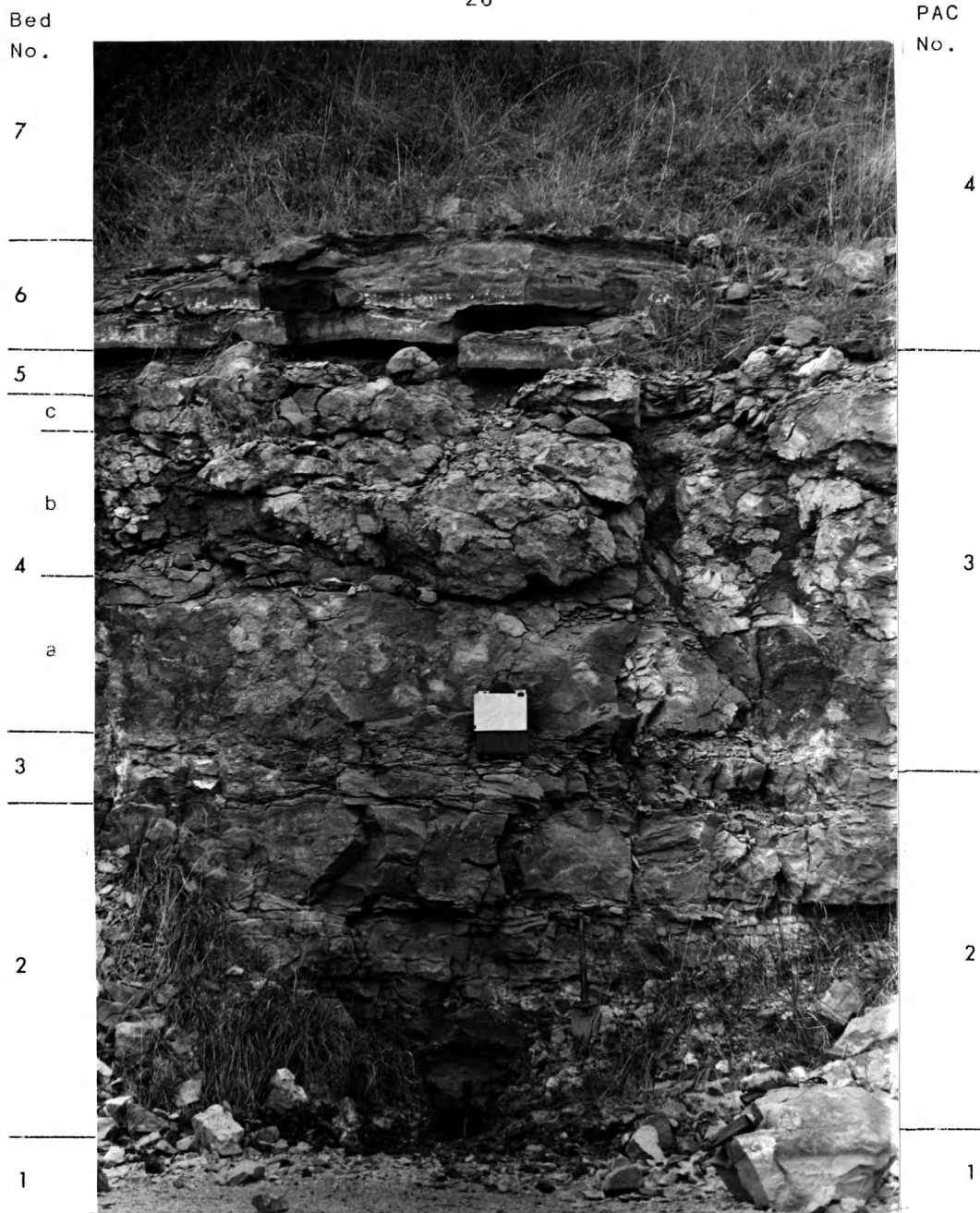
Figure 9. Overall outcrop at station 31, Locality 700. Hammer sits on top of Little Osage Shale at its contact with the Houx-Higginsville Limestone, which extends upward to where the soil and vegetation occurs. Base of clipboard is even with cherty layer in bed 3 (see stratigraphic section 700 in Appendix A, and section 31 in Appendix B). Hammer is approximately 31 cm long.
