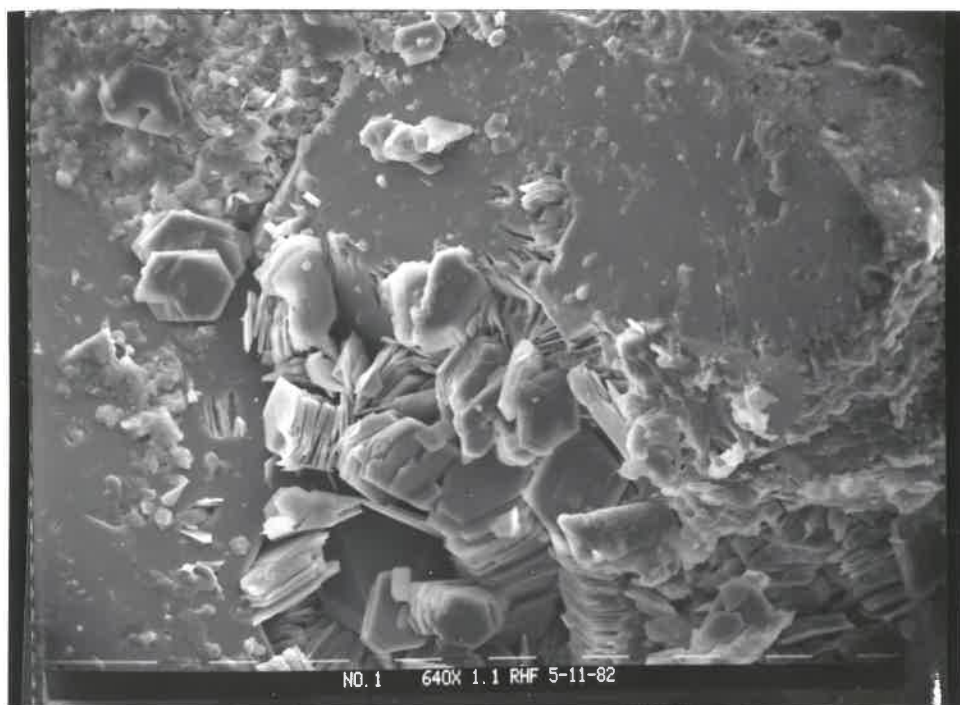
Fig. 32 SEM Photomicrograph - Authigenic kaolinite engulfed by quartz - lithofacies B. White bars = 10 microns.
