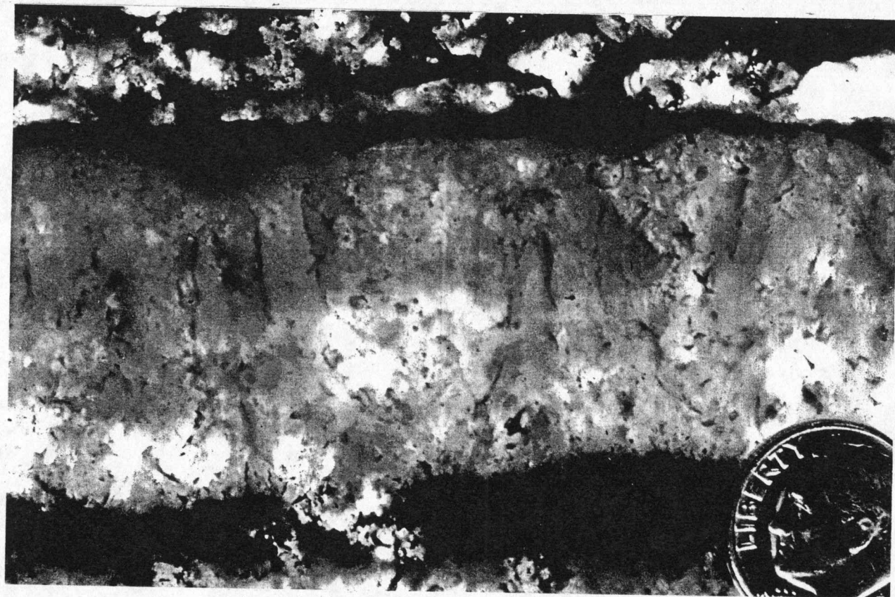
(951.5 FT) Plate 1 Samples 940 1-3, 290.2 m. Left photo; Partially recrystallized halite, vein of medium - coarse clear halite cross - cutting beds of chevron halite and clay - anhydrite laminations. Right photo; Chevron halite bed with small portions of intimately associated clear halite. The thin dark vertical lines are "walls" of clay and anhydrite which outline the chevrons. Coin is 0.68 IN in diameter.
