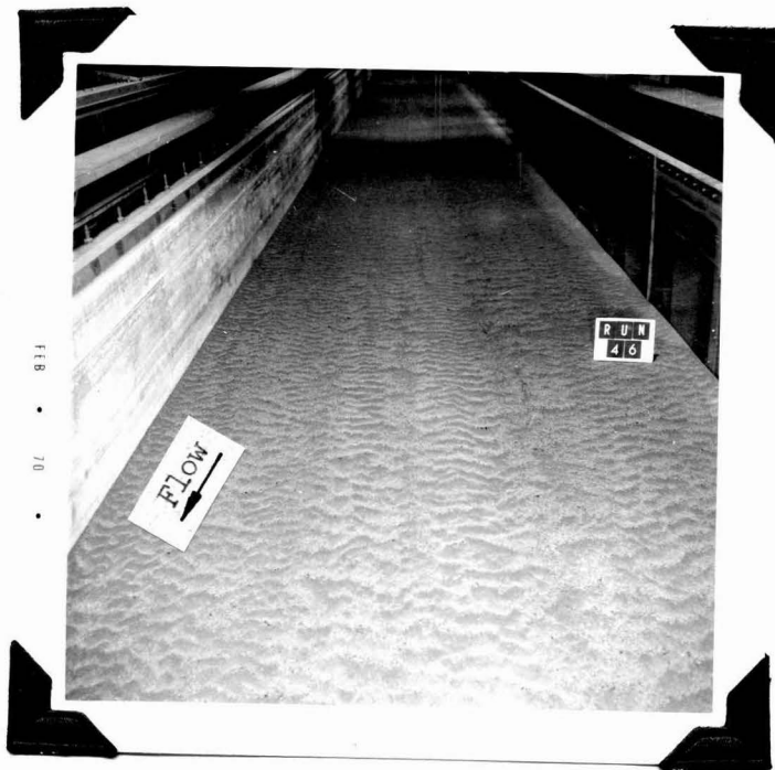
Fig. 21 Flat-bed surface (view upstream) formed by run 4. The sign represents continuous series number. Ripples at the surface were due to shut down of the flume.
