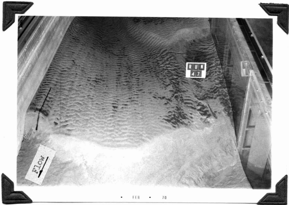
Fig. 15. Accumulations of dark opaque heavy minerals on the upstream sides of dunes (run 2). Location of cut-away view of dune (fig. 17) is shown by the line near the flume wall on left side of photo. The ripple surface that is shown on the dune is due to abrupt changes in hydraulic flow conditions that occurred when the flume was shut down at the end of the run.
