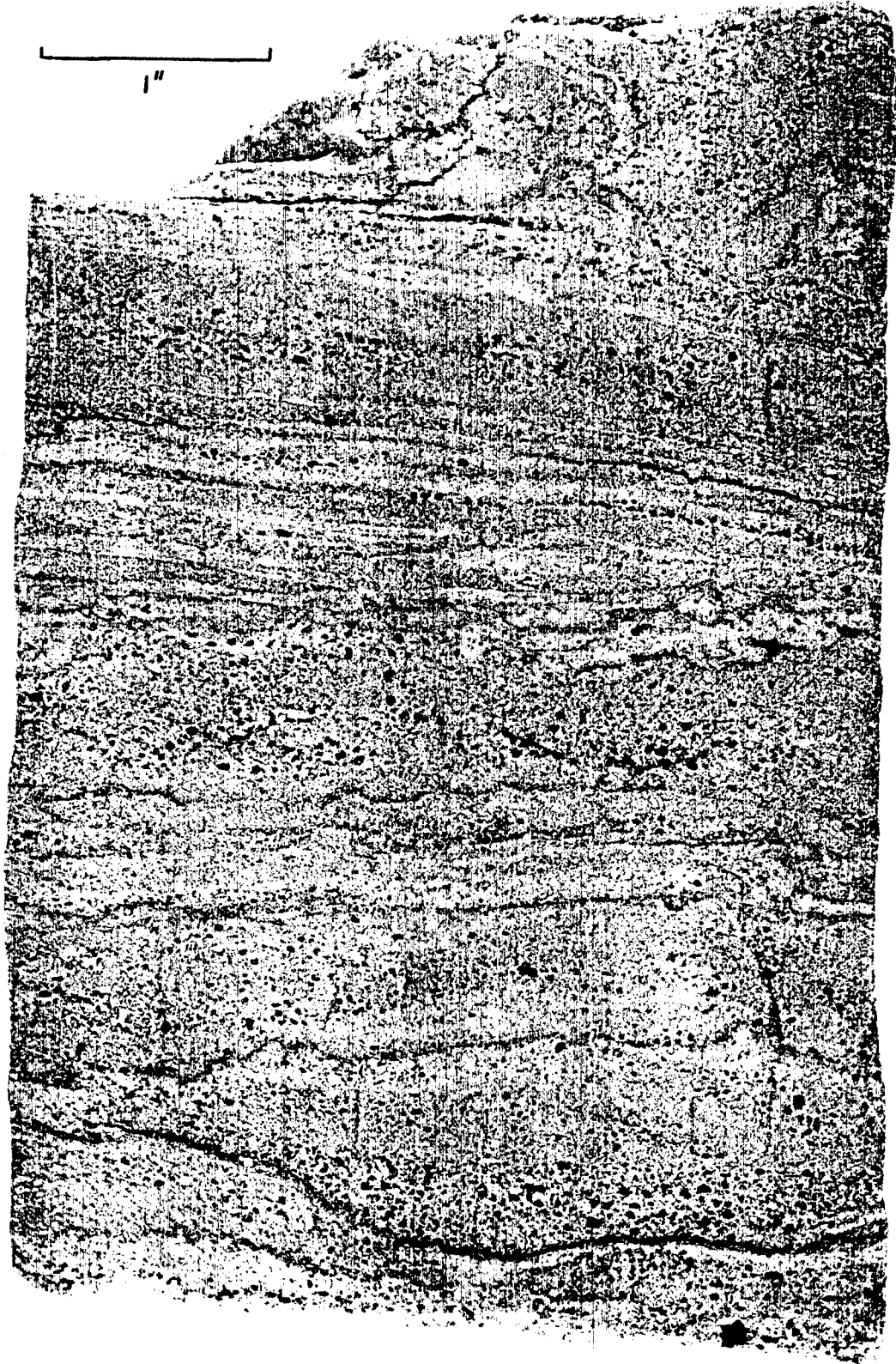
Figure 15.-Photograph of Reagan core from the Magnolia No. 1 "B" Holsman well, sec. 15, T 7 S, R 19 W, Rooks County, Kansas. Note size distribution of grains, illite laminae and irregular nature of illite layers (depth, 3535.6 to 3535 feet).
