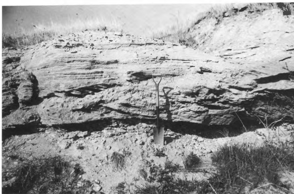
FIGURE 21. Crossbedded and cemented alluvial sand and gravel, tentatively assigned to the Ogallala Formation, in a quarry in the NE sec. 13, T. 14 S., R. 14 W.
