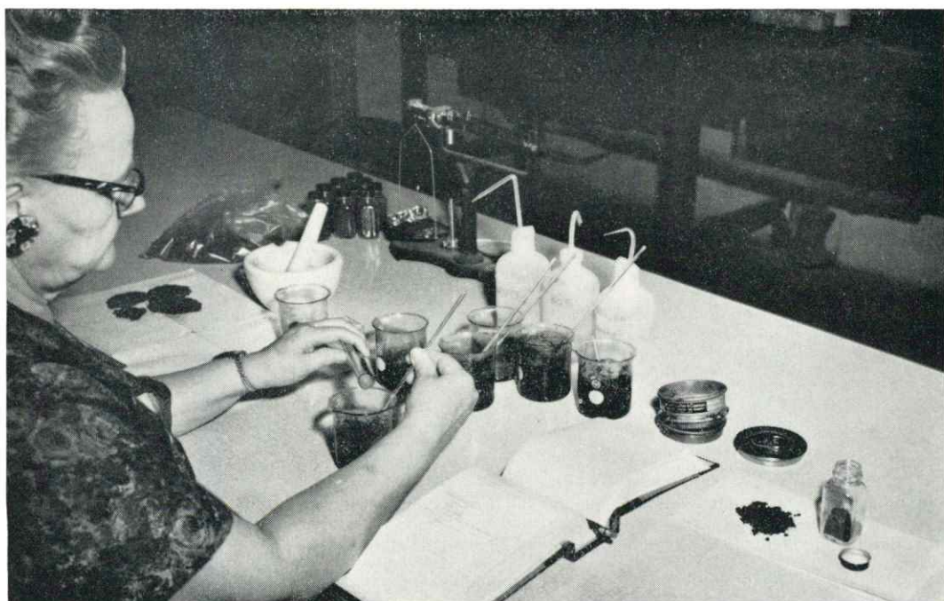
Lignite study. . . . Samples of lignite from central Kansas are being treated for production of humic acid to use as a soil conditioner.
