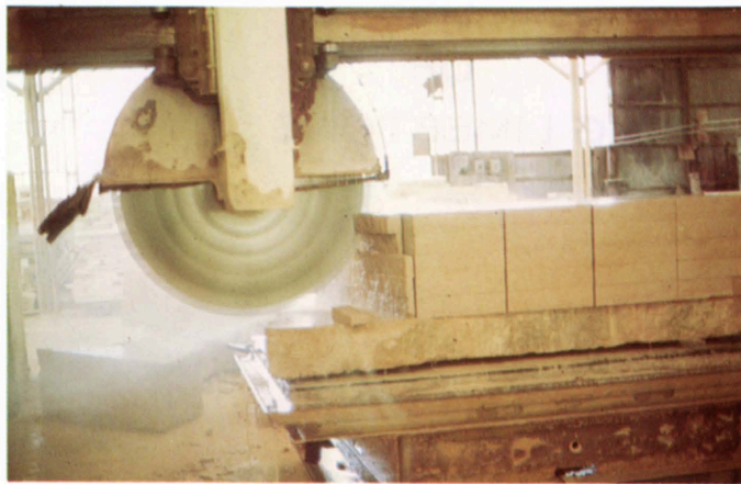
Fig. 9 - A diamond coated circular saw used to cut slabs. Water is used to facilitate cutting and control dust.
