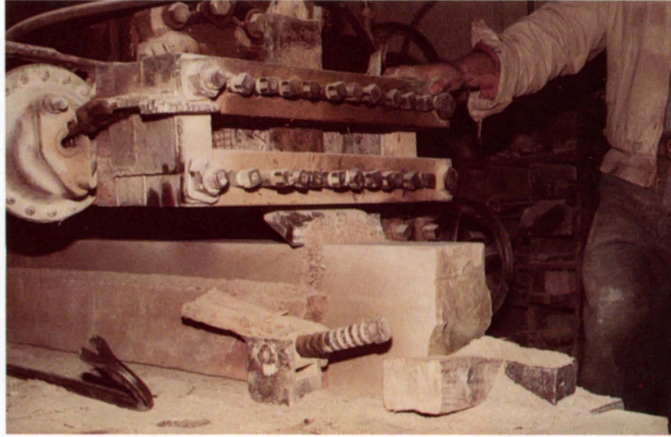
Fig. 11 - A planer adds the finishing touches to a surface to form a smooth face finish.
