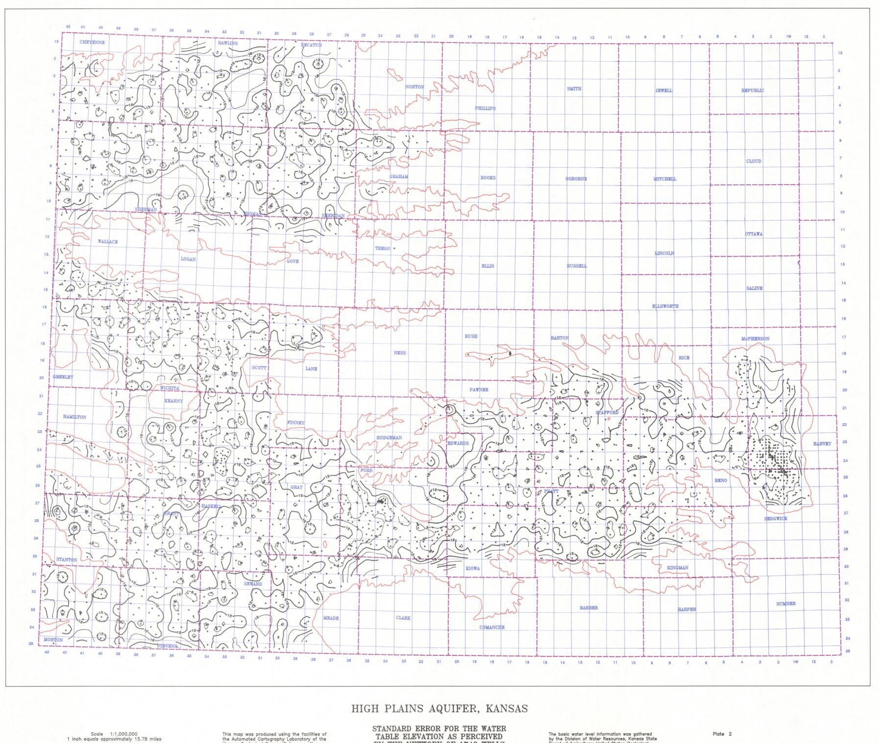
10 0 20 30 miles This map was produced using the facilities of the Automated Cartography Laboratory of the Kansas Geological Survey. Data correction, contouring and projection were performed by computer. Digitizing, editing and production of the reference geographical map were performed using the GIMMAP software developed jointly by the Kansas Geological Survey and the Bureau de Recherches Geologiques et Minieres, Orleans, France. Minieres, Orleans, France.
