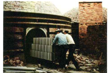
Raw tile being wheeled into a kiln for firing.
