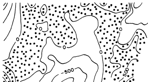
B. Arbitrary: Trend = -1897 + 2457X - 515.5Y - 13,213\text{LOG}X + 2342\text{LOG}Y . 84.4% sum of squares accounted for by trend. Condition value of R matrix = 4.0 \times 10^{-4} .
