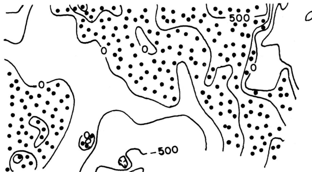
A. Quadratic: Trend = 1237 - 2179X + 280.9Y + 404.5X^2 + 29.41XY - 82.12Y^2 . 83.7% sum of squares accounted for by trend. Condition value of R matrix = 8.6 \times 10^{-6} .
