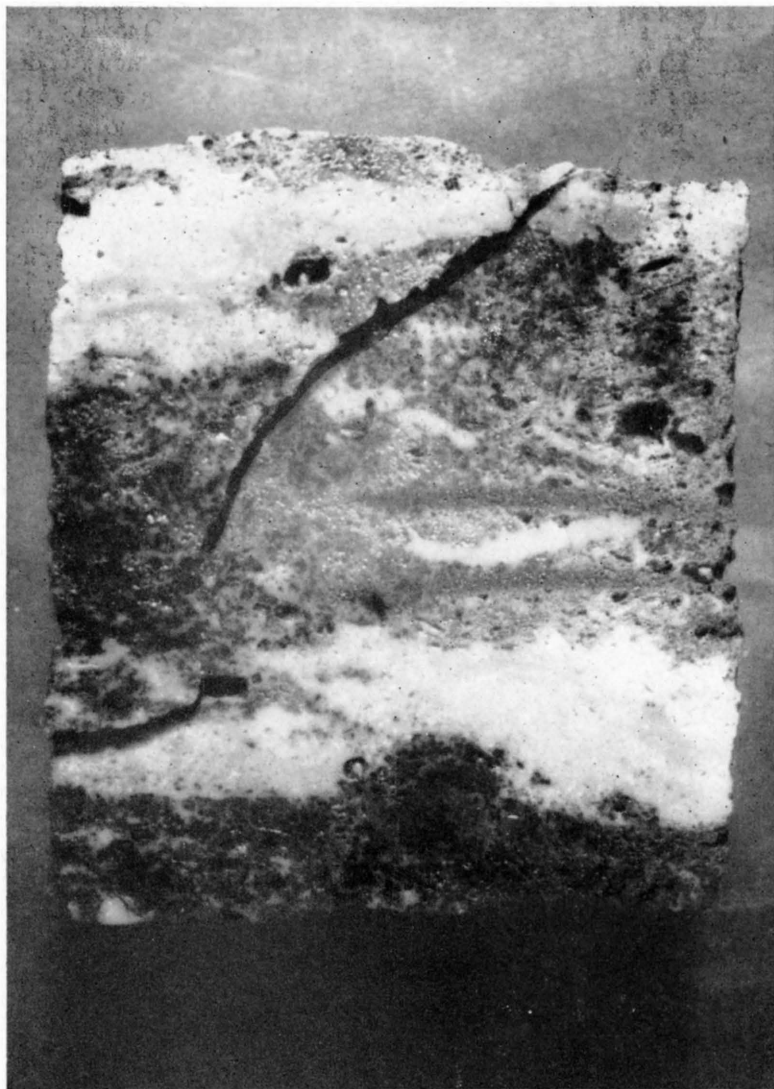
PLATE 6. Photograph of core, sawed in half, (X 1\frac{1}{4} ) from dolomite yielding oil in undifferentiated Burlington and Keokuk limestones of Mississippian age. The core was taken at 1,595 feet in J. B. Apperson et al. (T. W. Sowell) No. 1 Bower well, in the SE \frac{1}{4} NE \frac{1}{4} sec. 5, T. 10 S., R. 20 E.
