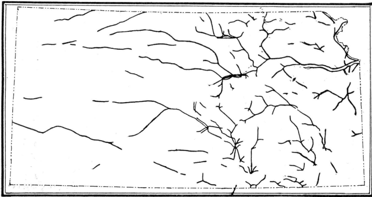
FIGURE 16. Map showing the railroads in Kansas which are laid in river valleys. River valleys are natural highways, which even in plains country like Kansas control largely the position of railroads and the location of cities.
