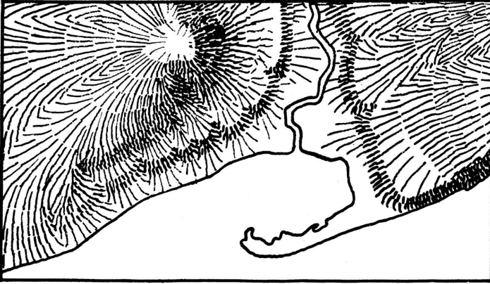
FIGURE 37. Hachure map of area shown in Figure 34. The direction of slope is indicated by the direction of the lines, the steepness of slope by the weight and crowding of the lines. Hachure maps are employed by the French general staff.
