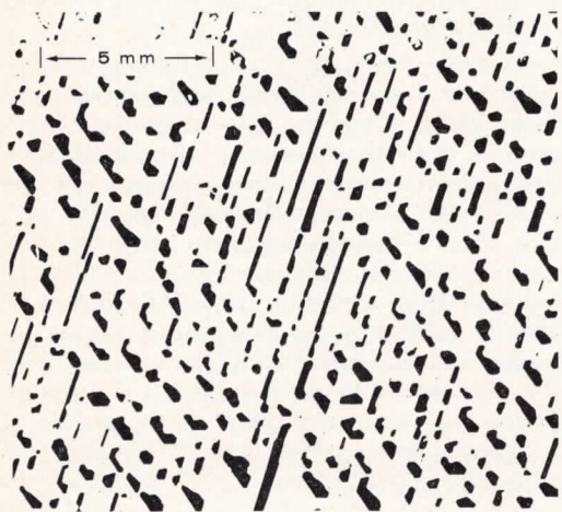
FIGURE 5.—Photomicrograph of a pyroxene-ilmenite intergrowth from the Monastery Mine kimberlite, South Africa (after Dawson and Reid, 1970).
