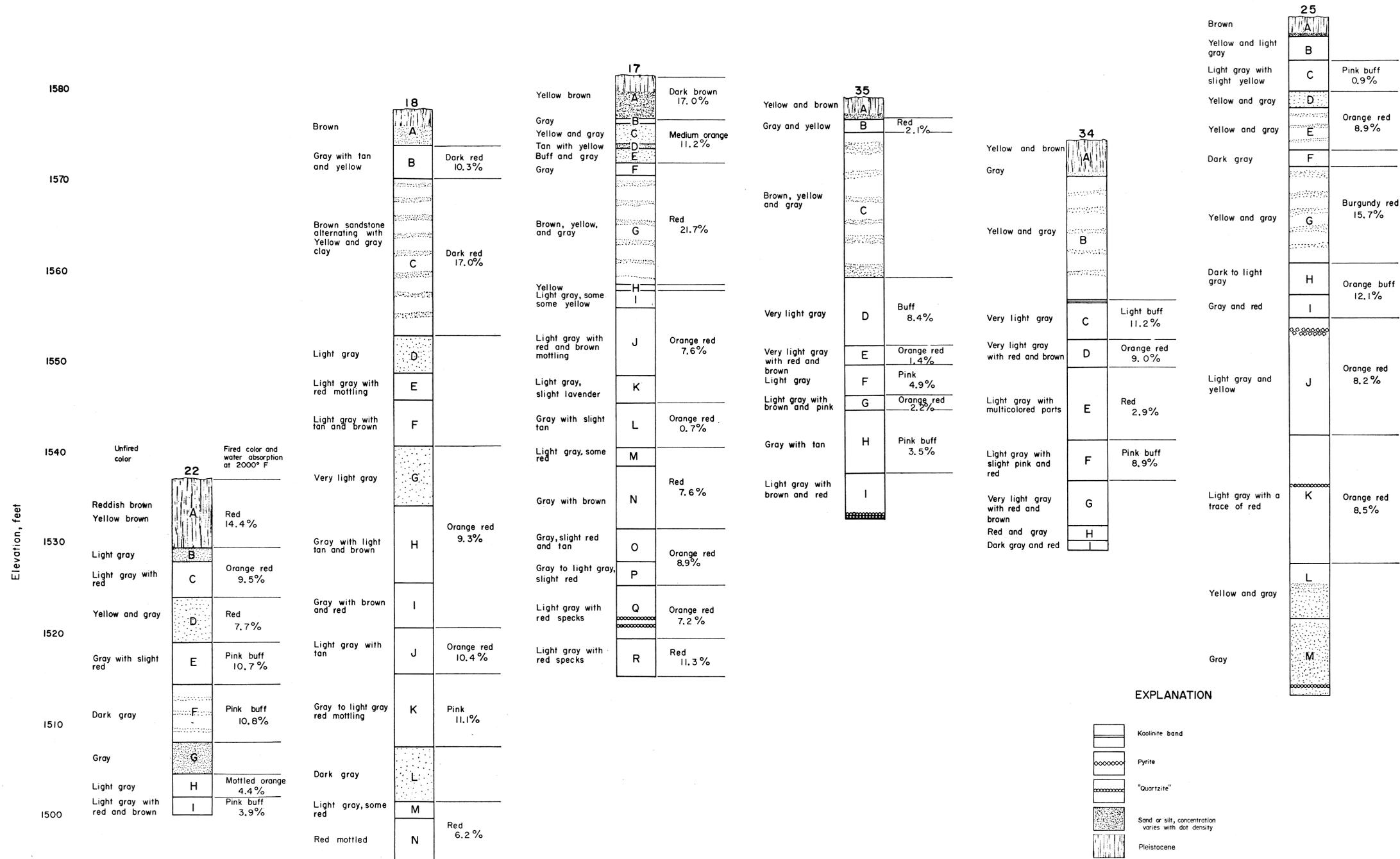
FIGURE 4.—Graphic logs of selected test holes in C-12 area. (Locations of test holes shown on Figure 2; for test-hole numbers, see Appendix, Cloud County.)
