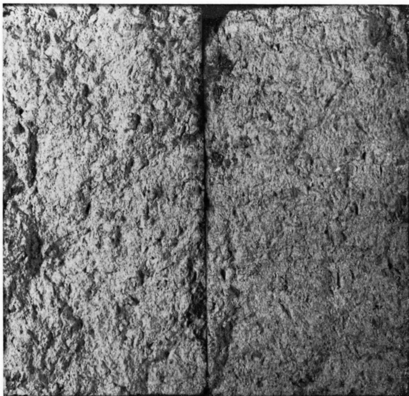
PLATE 8.—Broken brick L-39-2, medium texture, modulus of rupture 750 psi.
