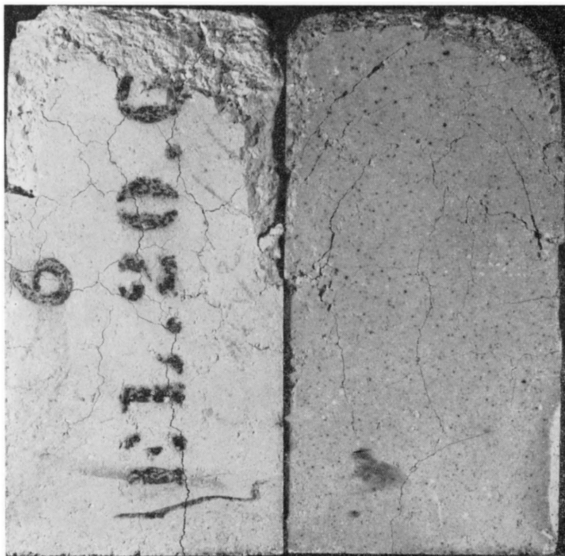
PLATE 6.—High-silica-content bricks showing thermal shock induced by load-test heating.
