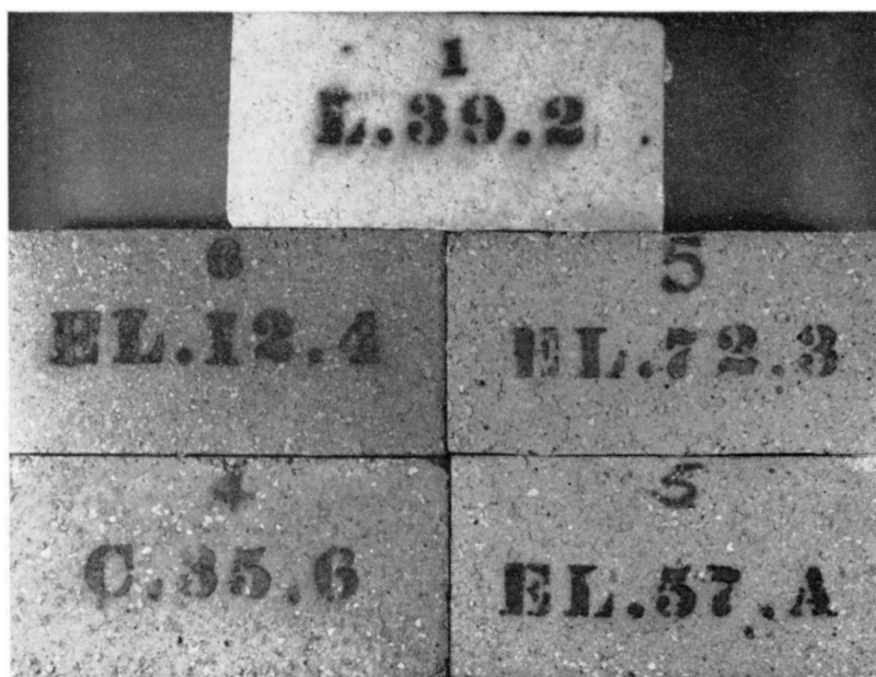
PLATE 4.—Bricks having acceptable handling strength after hot load testing.
