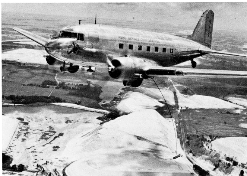
FIG. 4.—The aircraft in which amplifiers and recording elements are mounted and the towed "bird" of the airborne magnetometer.
