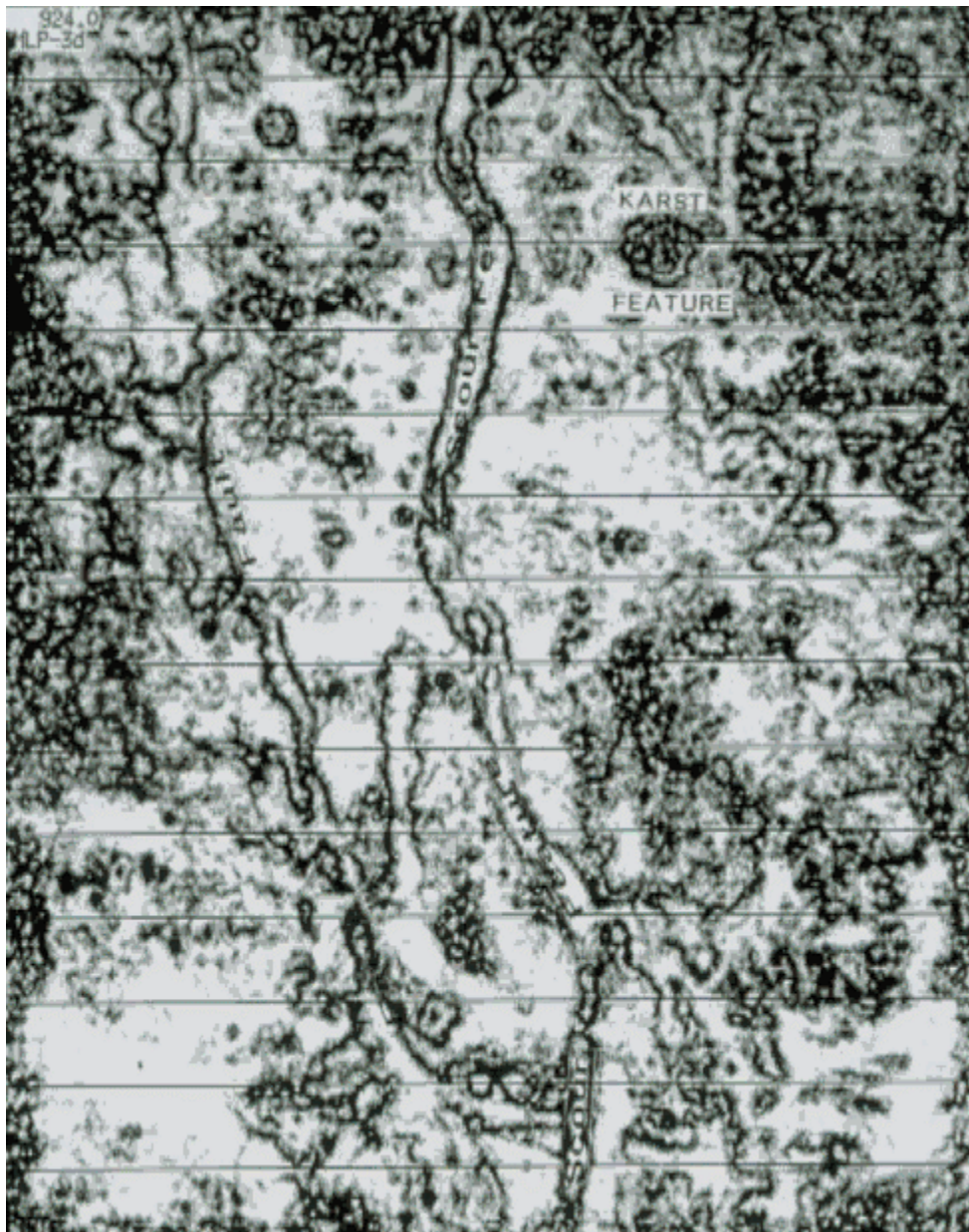
Figure 5. Seismic coherence time slice at 924 ms through the South Eubank Field 3-D seismic survey, showing a regional fault, a major Chester scour feature, and a karst feature.
