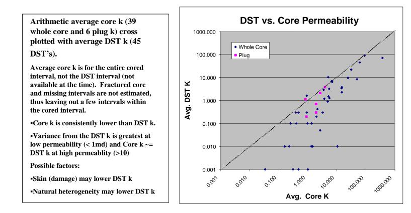
Figure 9.2.8. Comparison of permeability from drill-stem tests with that from Chase and Council Grove core from multiple wells in Stevens County, Kansas.
