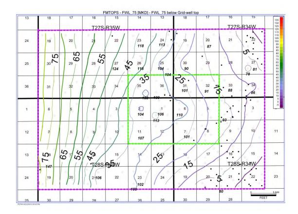
**Figure 9.4.5.** Structure on the free-water-level (FWL) surface, datum is sea level. Elevation of lowest perforation in Council Grove is posted by well spots where available. Elevation of FWL surface = (Elevation of lowest Council Grove perforations -75 ft).
