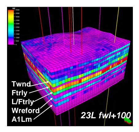
Figure 9.4.6. Original-gas-in-place (OGIP) charging the Graskell model that served as the basis for reservoir simulation studies.
