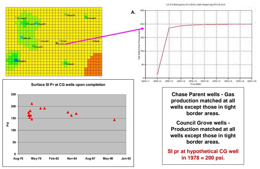
**Figure 9.4.44.** RUN 10 Results – A) Simulator-calculated shut-in pressure at a hypothetical Council Grove well completed in January 1978.
