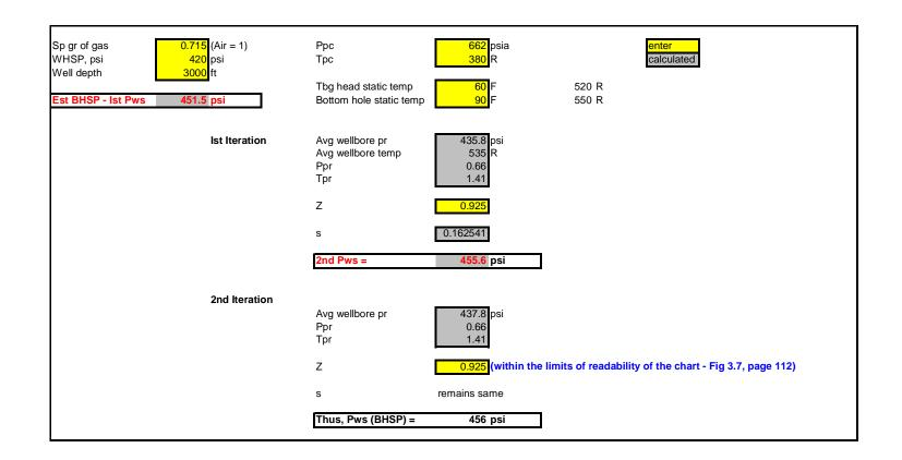
Figure 9.2.11. Calculation process to convert surface shut-in pressure to bottom-hole shut-in condition.
