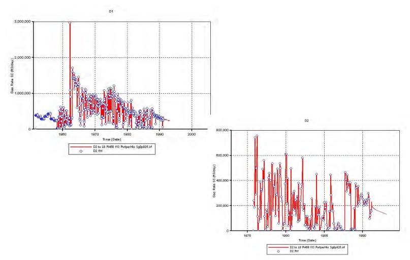
Figure 9.2.19. RUN 4 Results - Simulator-calculated flow rates at D1 and D2 wells compared with historic volumes.
