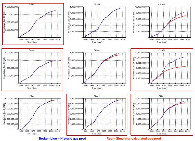
**Figure 9.4.21.** RUN 4 Results – Simulator-calculated cumulative gas production compared with historic production for Chase Parent wells.
