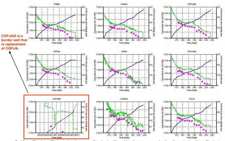
Red line – Simulator (Sim) calculated cum gas, Blue broken line – historic cum gas production, Green broken line – Sim bottom hole pressure (BHP flowing), Magenta circles – Well head flowing pressure (WHFP).
