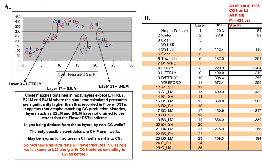
**Figure 9.3.38.** RUN 6 Results – A) Simulator calculated layer pressure at Flower A1 compared with layer DST pressure. B) Tabulation of simulator-calculated layer pressure with that obtained from Flower well DSTs.
