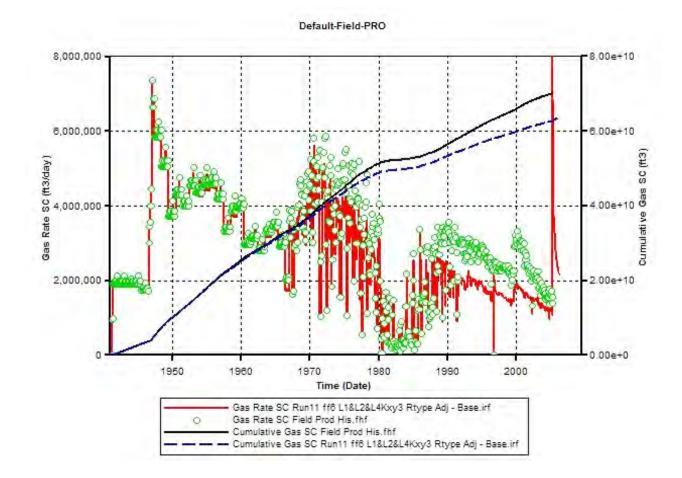
**Figure 9.5.32.** RUN 5 Results – Simulator-calculated cumulative production and production rate from the Hoobler study area compared with historic volumes.
