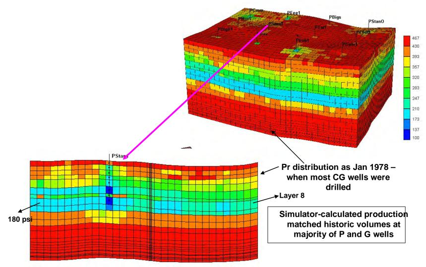
**Figure 9.4.32.** RUN 9 Results – Simulator-calculated pressure distribution as of January 1978 after which majority of Council Grove wells came online.
