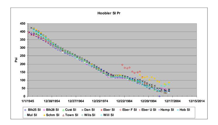
Figure 9.5.13. Plot of surface shut-in pressures at Chase wells in the Hoobler area over time.
