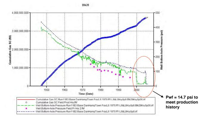
Figure 9.5.41. RUN 9 Results – Cumulative production and flowing-pressure history match at well Blk28.
