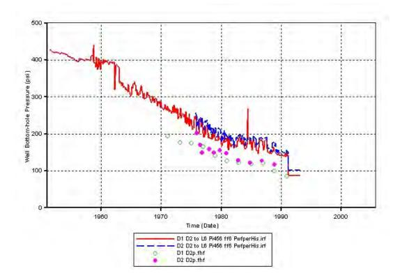
**Figure 9.2.17.** RUN 2 Results - Simulator-calculated bottom-hole flowing pressure at D1 and D2 wells compared to corresponding historic values show presence of excess flow capacity.
