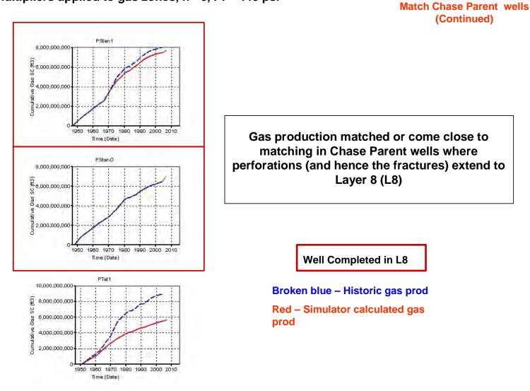
**Figure 9.4.14.** RUN 1 Results – Simulator-calculated cumulative gas production compared with historic production for Chase Parent wells.
