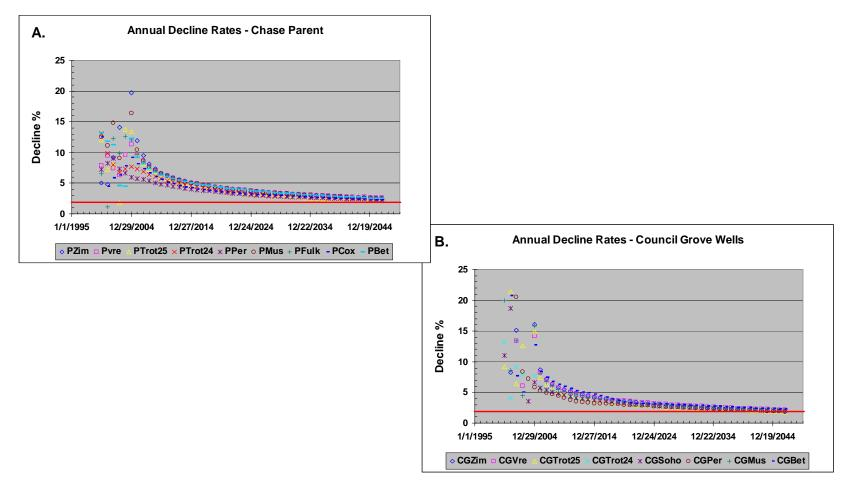
**Figure 9.3.44.** RUN 7 Results – Simulator-calculated annual production decline rates in Chase Parent and Council Grove wells till 2050.
