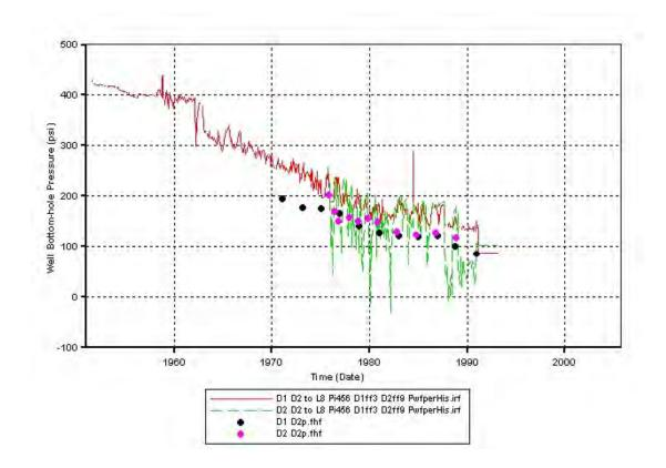
**Figure 9.2.25.** RUN 7 Results - Simulator-calculated bottom-hole flowing pressure at D1 and D2 wells compared to corresponding historic values recorded at the surface.
