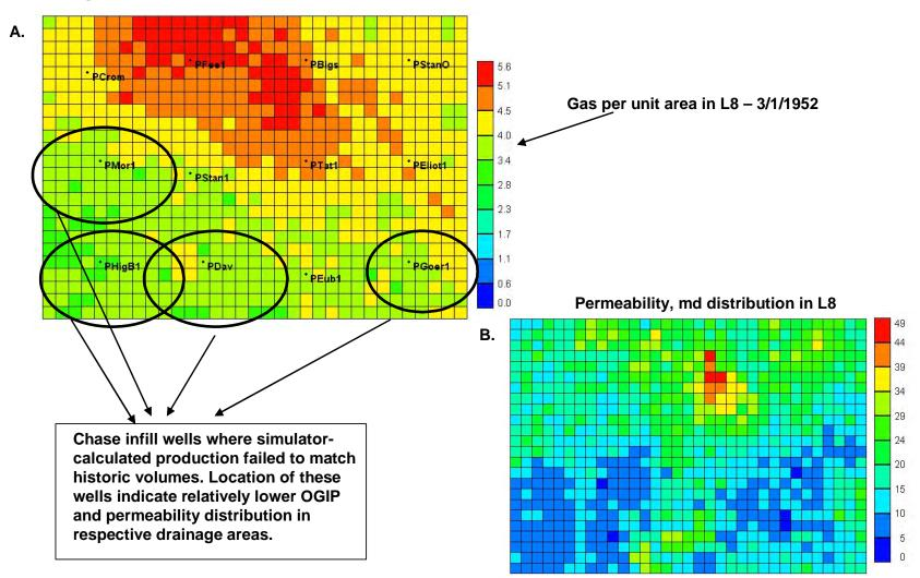
**Figure 9.4.43.** A) Location of Chase Infill wells where simulator-calculated production failed to match historic volumes. B) Permeability distribution in Layer 8 (one of the main driver zones) shows tight permeability along the southern part of the study area.
