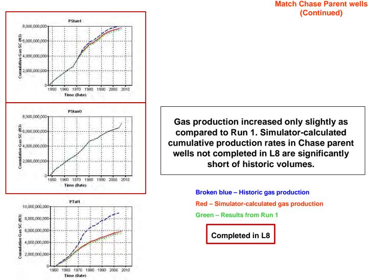
**Figure 9.4.18.** RUN 2 Results – Simulator-calculated cumulative gas production compared with historic production for Chase Parent wells.
