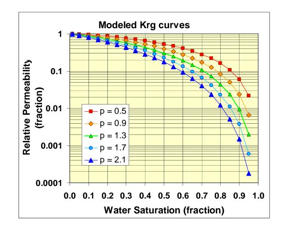
Figure 9.1.8. Range of possible gas relative-permeability values for first and second standard deviation.
