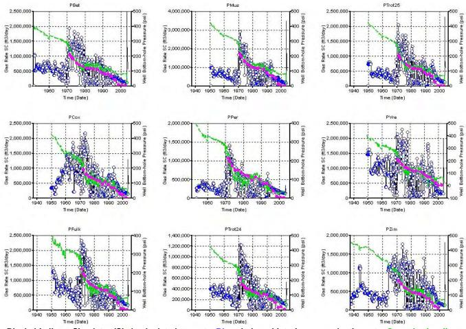
Black thin line – Simulator (Sim) calculated gas rate, Blue circles – historic gas production rate, Green broken line – Sim bottom hole pressure (BHP flowing), Magenta circles – Well head flowing pressure (WHFP).
