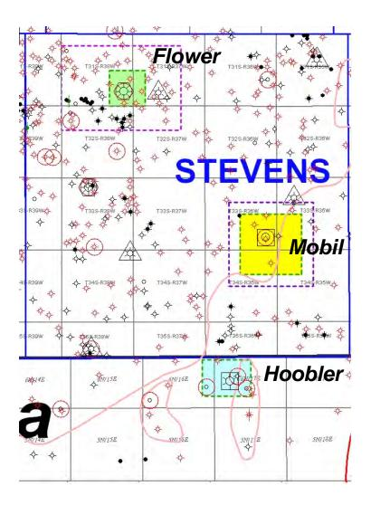
**Figure 9.5.3.** Map showing node wells in and around the Hoobler study area that were used in Geomod 4 to build a full-field model. Wells with pressure data are shown circled.
