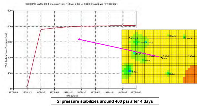
**Figure 9.4.33.** RUN 9 Results – Simulator-calculated shut-in pressure at a hypothetical Council Grove well completed in January 1978.
