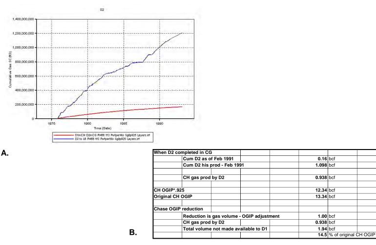
**Figure 9.2.21.** RUN 5 Results – A) Simulator-calculated cumulative production from D2 with its completion restrained within Council Grove (red line) compared with that when its completions extended to Towanda in Chase (blue line). B) Calculation showing volume of Chase gas that was not available to D1 well for production.
