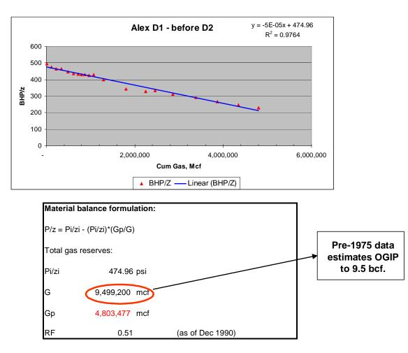
**Figure 9.6.3.** Plot of P/z vs. Gp data from Alexander D1 until 1975, and original-gas-in-place calculation from the materialbalance plot.
