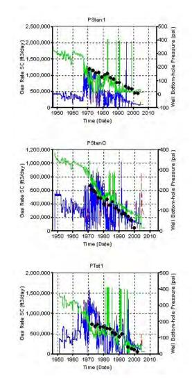
Final history matches – CH P wells Production matched at all but PHigB1 Pressure matched at few wells Pressure spikes indicate tight K Production spikes when released of flow constraints
