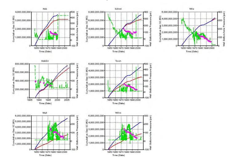
Figure 9.5.20. RUN 1 Results – Cumulative production- and pressure-history matches obtained at the Chase wells.
