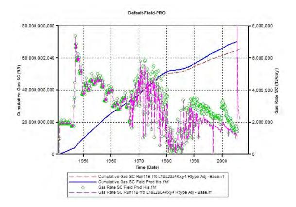
**Figure 9.5.34.** RUN 7 Results – Simulator-calculated cumulative production and production rate from the Hoobler study area compared with historic volumes.
