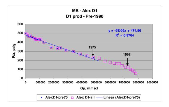
Figure 9.6.4. Plot of P/z vs. Gp data from Alexander D1 until 1990.
