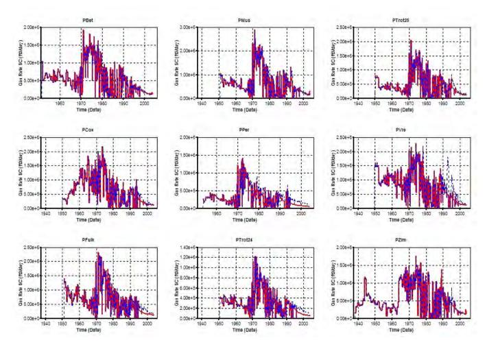
**Figure 9.3.27.** RUN 5 Results – Comparison of simulator-calculated production rate with historic values at Chase Parent wells when completions in Council Grove wells extended to Layer 2 and initial reservoir pressure is assumed to be 423 psi.
