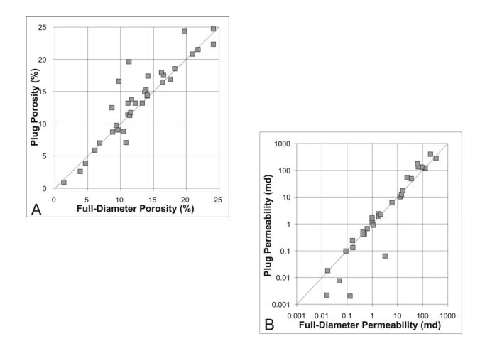
**Figure 9.3.10**. Crossplot of full-diameter core porosity versus plug porosity (A) and permeability (B) for samples in which the fulldiameter cores did not exhibit any apparent microfracturing. Good correlation indicates that matrix-scale properties apply to fulldiameter scale. Variance can be attributed to full-diameter core sampling multiple lithoface or a range in porosity not sampled by the corresponding core plug.
