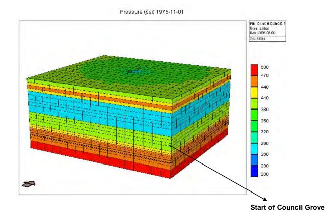
**Figure 9.2.15.** RUN 1 results – Simulator-calculated pressure distribution in the study area as of November 1975 as a result of production from D1 shows differential depletion.
