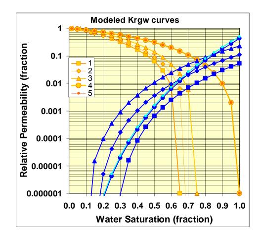
Figure 9.1.7. Gas and water relative-permeability curves for different rock-types.
