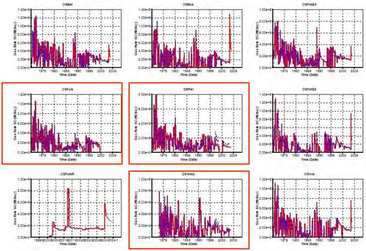
Red line - Simulator (Sim) calculated gas rate, Blue broken line - historic gas production rate
