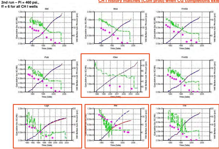
Red line – Simulator (Sim) calculated cum gas, Blue broken line – historic cum gas production, Green broken line – Sim bottom hole pressure (BHP flowing), Magenta circles – Well head flowing pressure (WHFP).
