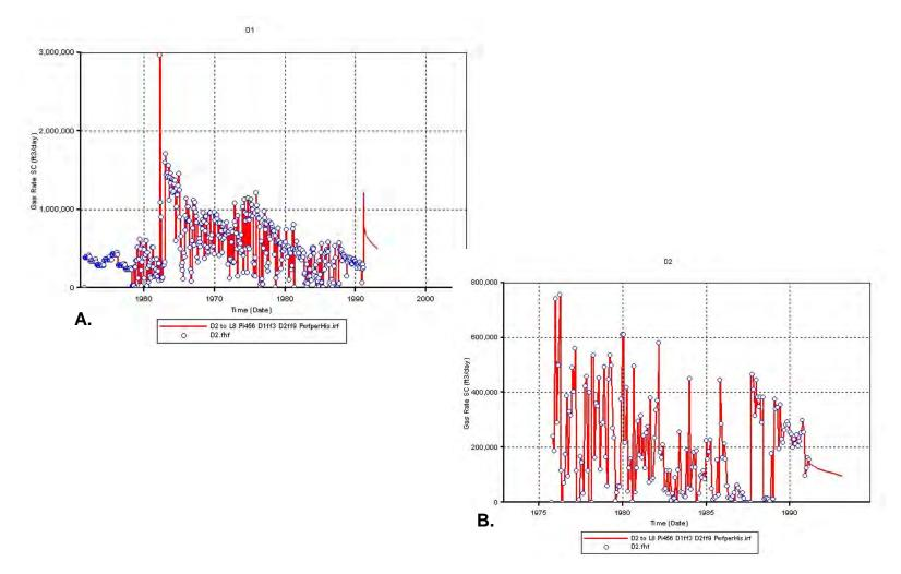
Figure 9.2.24. RUN 7 Results - Simulator-calculated flow rates at D1 and D2 wells compared with historic volumes.
