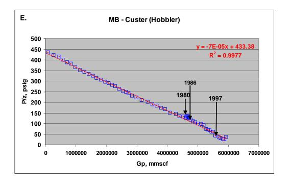
MB trend line indicates that something taking place at the well near 1979 that resulted in a loss of linearity of the P/z vs. Gp data.
