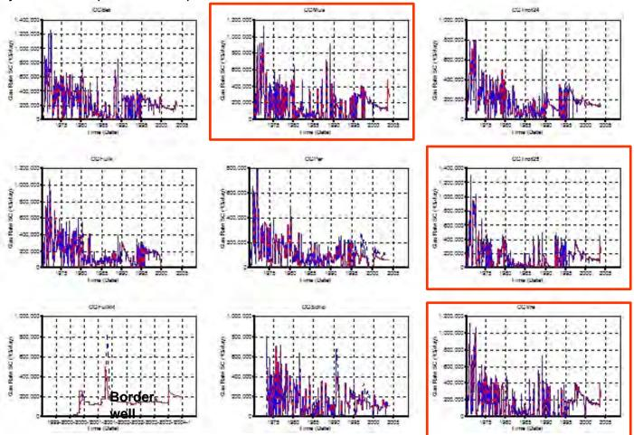
**Figure 9.3.31A.** RUN 6 Results – Comparison of simulator-calculated production rate with historic values at Council Grove wells when Council Grove completions extended to Layer 2, initial reservoir pressure set to 423 psi, and ff adjusted in CH P and CG wells.
