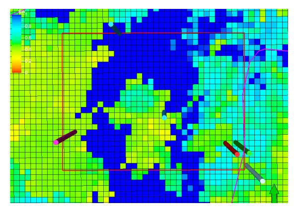
**Figure 9.5.5.** Map view of water saturation for top layer in the Herington in Geomod4. Outline of Hoobler area is marked in red. Wells shown are the model "node" wells with qualified log data.
