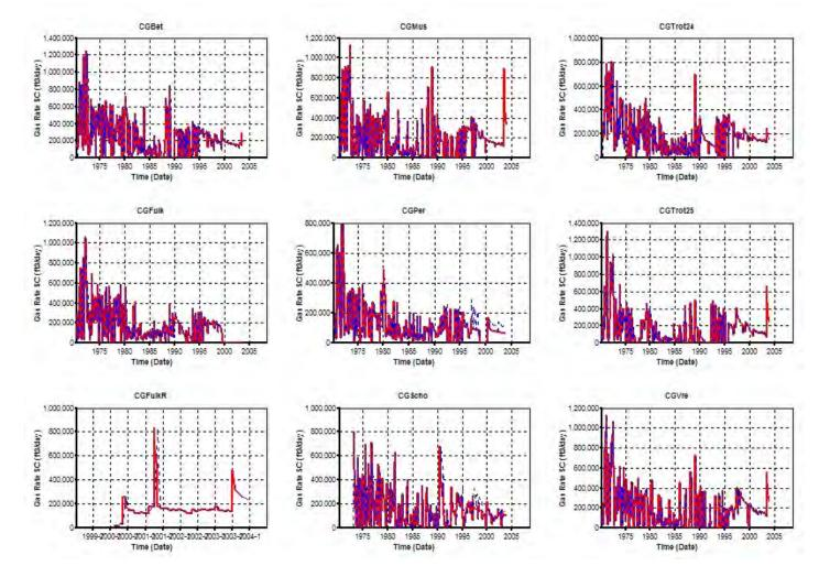
**Figure 9.3.28A.** RUN 5 Results – Comparison of simulator-calculated production rate with historic values at Council Grove wells when completions in Council Grove wells extended to Layer 2 and initial reservoir pressure is assumed to be 423 psi.
