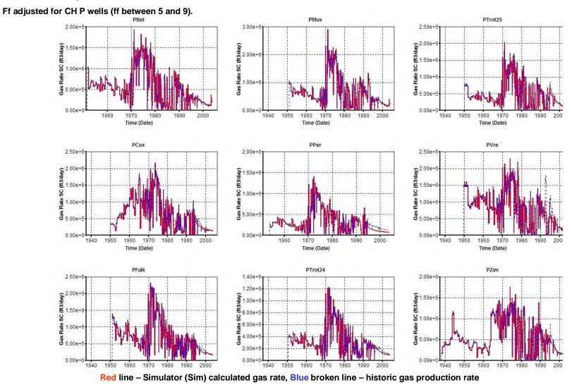
**Figure 9.3.23.** RUN 3 Results – Comparison of simulator-calculated production rate with historic values at Chase Parent wells when completions in Council Grove wells extended to Layer 2 and initial reservoir pressure is assumed to be 435 psi.
