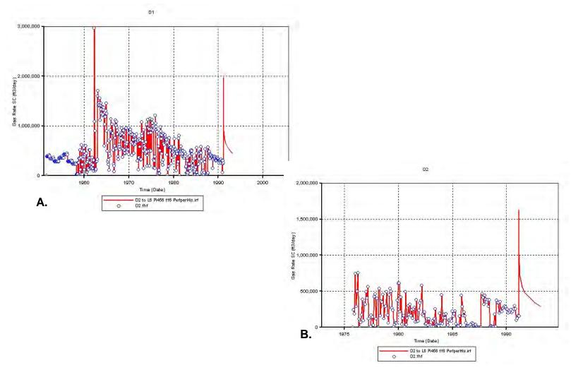
Figure 9.2.16. RUN 2 results - Comparison of simulator-calculated production (line) from D1 (A) and D2 (B) with their respective historic rates (points).
