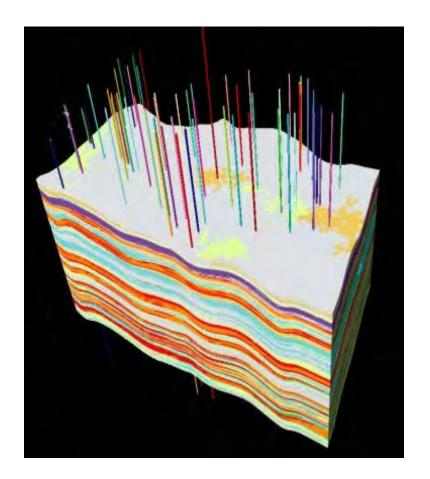
**Figure 9.3.4.** 234-layer 3D volume of static model showing (color-coded) lithofacies in the 70 square mile around the Flower study area. Wells with facies and porosity information are shown (node wells).
