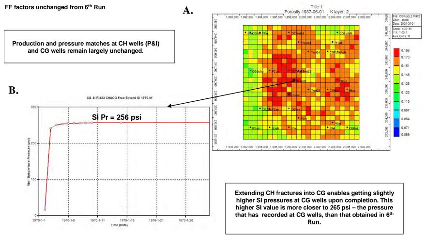
**Figure 9.3.39.** RUN 7 Results – Chase wells completions extended to Layer 23 while Council Grove completions extended to Layer 2. A) Relative location of hypothetical Council Grove well in the Flower study area. B) Simulator-calculated shut-in pressure at the hypothetical Council Grove well as of January 1970.
