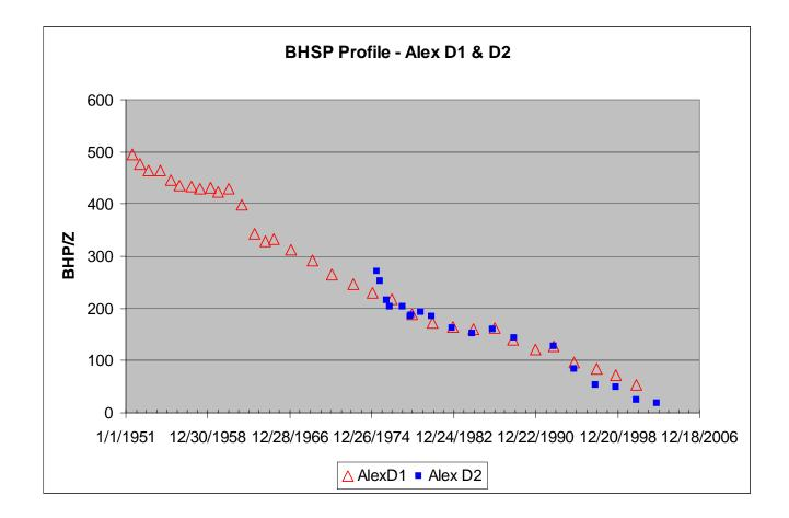
**Figure 9.2.2.** Plot comparing bottom hole shut-in pressures recorded at D1 and D2. Overlap of pressures indicative of communication between Chase and Council Grove reservoirs.
