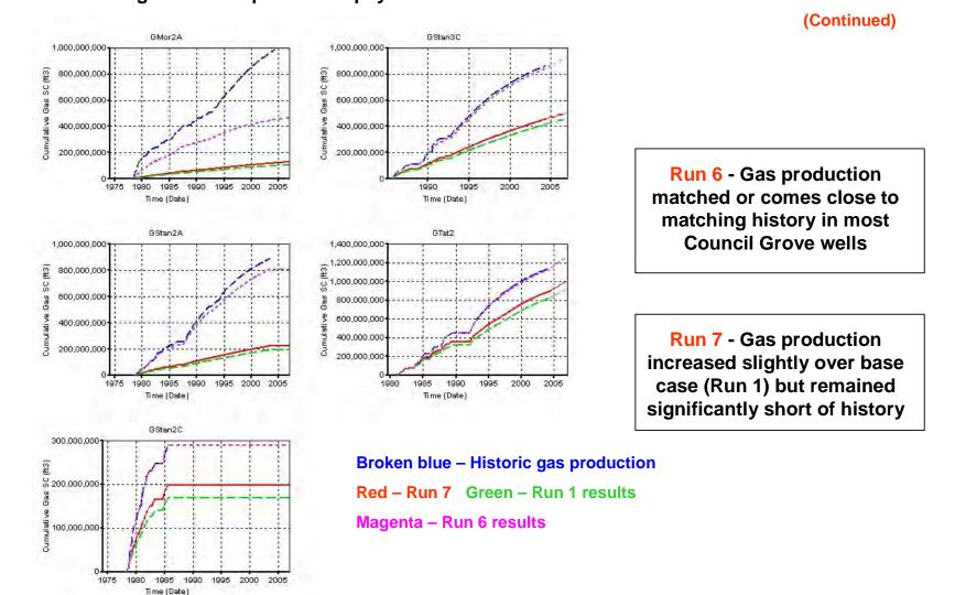
**Figure 9.4.29.** RUN 6 and 7 Results – Simulator-calculated cumulative production at Council Grove wells compared with historic values.
