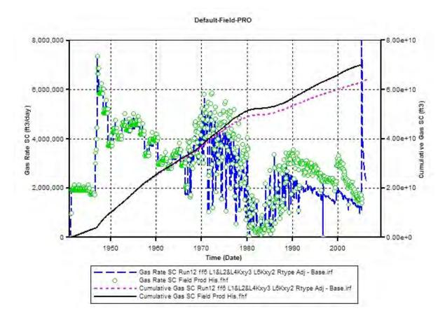
**Figure 9.5.33.** RUN 6 Results – Simulator-calculated cumulative production and production rate from the Hoobler study area compared with historic volumes.
