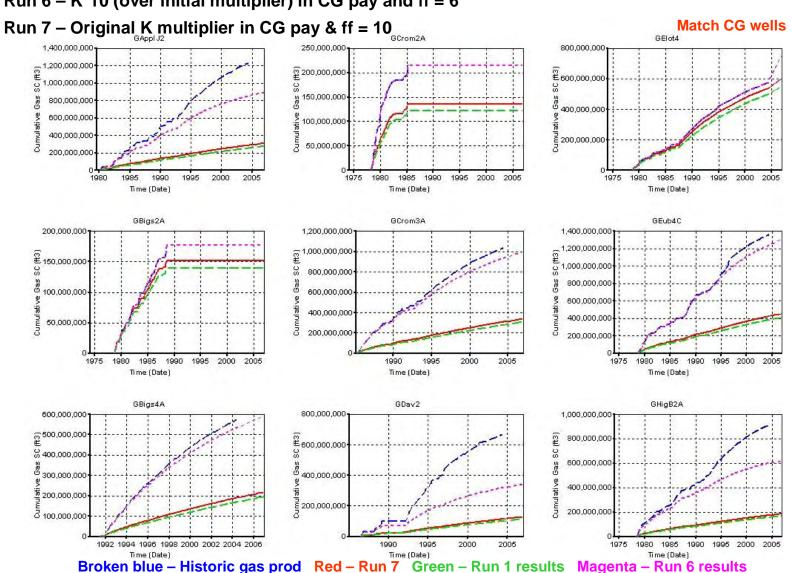
**RUNS 6 and 7:** Initial Kxy in Chase (as Run 3). Fractures constrained to perfs in CG. Pi = 440 psi Run 6 – K\*10 (over initial multiplier) in CG pay and ff = 6
