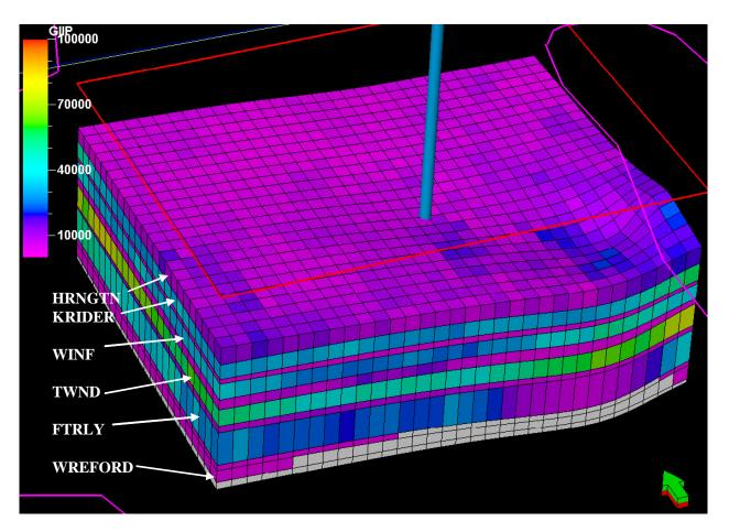
**Figure 9.5.7.** Distribution of gas-in-place (GIP) for the 11-layer model with a FWL at +65 ft above sea level. Hoobler well bore is shown located in the middle of the study area.
