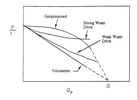
**Figure 9.6.1.** Expected profiles of P/z vs. Gp curves for reservoirs producing under different drive mechanisms from Lee and Wattenbarger, 1996, p. 236.
