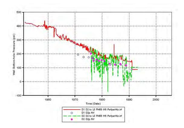
**Figure 9.2.23.** RUN 6 Results - Simulator-calculated bottom-hole flowing pressure at D1 and D2 wells compared to corresponding historic values recorded at the surface.
