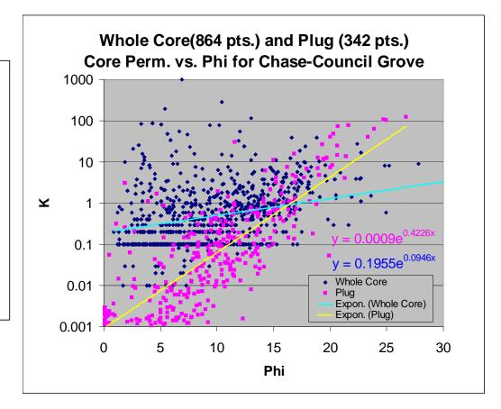
Figure 9.2.4. Comparison of permeability-porosity recorded on plugs and whole cores from Chase and Council Grove intervals.
