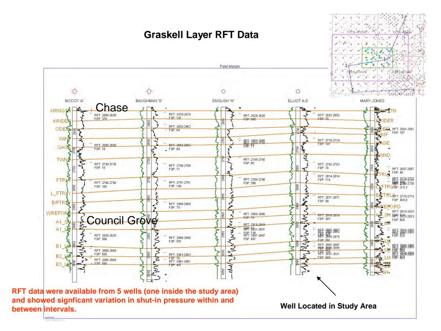
Figure 9.4.26. Cross section and map showing location of wells with RFT data in and around the Graskell study area.
