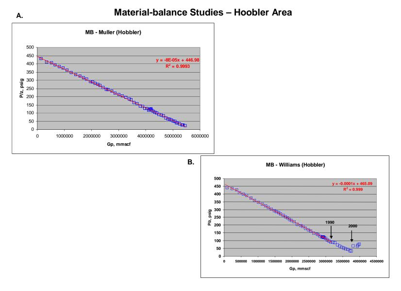
Figure 9.6.14. A) P/z vs. Gp plot for Muller well in the Hoobler study area. B) P/z vs. Gp plot for Williams well in the Hoobler study area.
