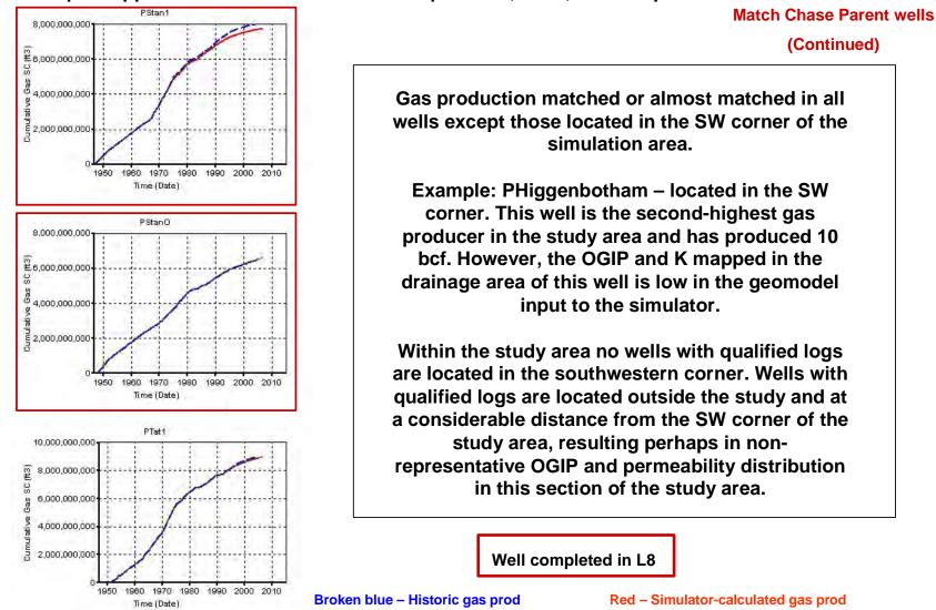
**Figure 9.4.22.** RUN 4 Results – Simulator-calculated cumulative gas production compared with historic production for Chase Parent wells.
