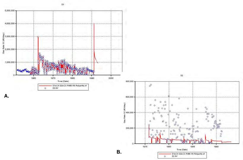
**Figure 9.2.14.** RUN 1 results – Comparison of simulator-calculated production (line) from D1 (A) and D2 (B) with their respective historic rates (points).
