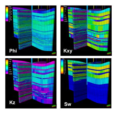
**Figure 9.5.6.** Porosity, permeability, and water saturation upscaled from 269 layers to 24 layers, one layer per zone in the Chase and Council Grove.
