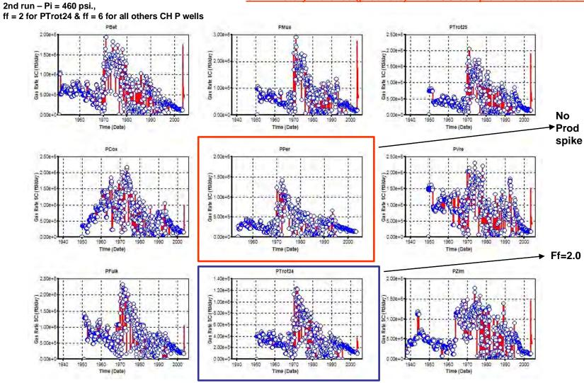
Red line – Simulator (Sim) calculated gas rate, Blue circles – historic gas production rate,
