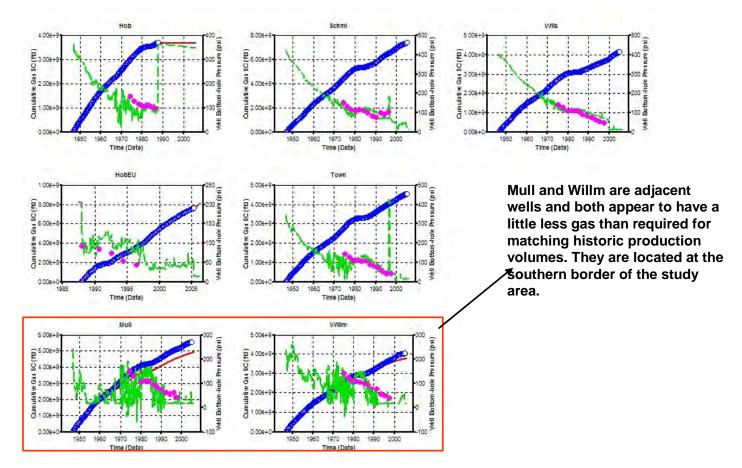
Figure 9.5.44. RUN 10 Results – Cumulative production and flowing-pressure history matches at Chase wells.
