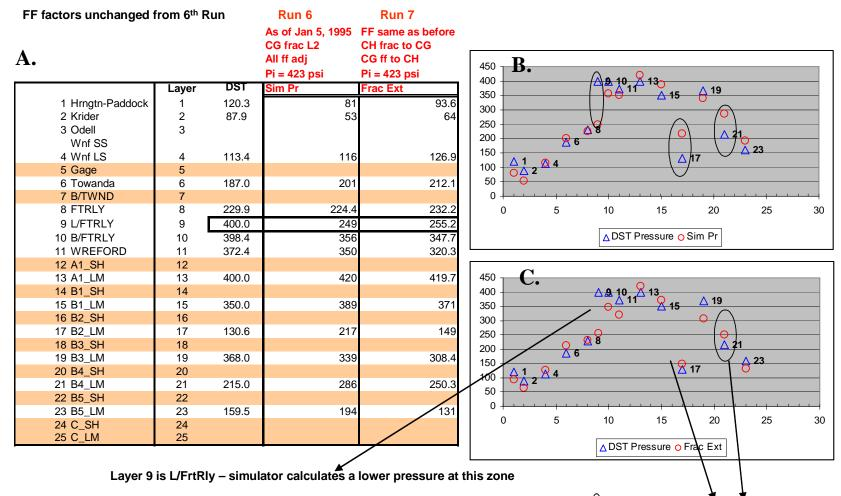
Pressure matches improve in Layers 17 and 21 when CH completions extended in CG
