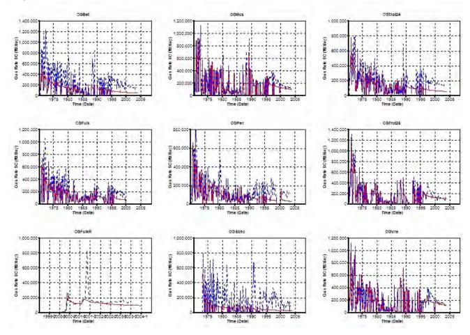
Red line – Simulator (Sim) calculated gas rate, Blue broken line – historic gas production
