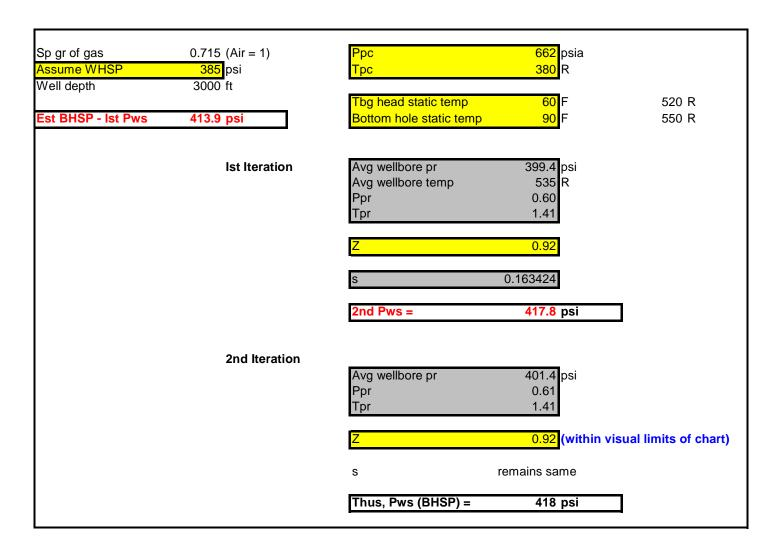
Figure 9.3.14B. Procedure to calculate bottom-hole shut-in pressure from well head shut-in pressure.
