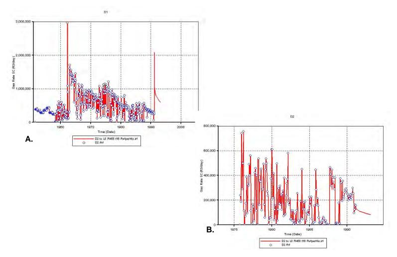
Figure 9.2.22. RUN 6 Results - Simulator-calculated flow rates at D1 and D2 wells compared with historic volumes.
