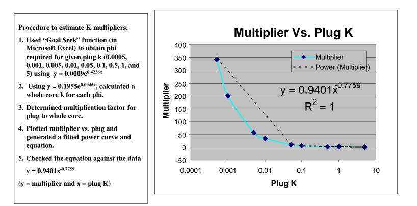
Figure 9.2.5. Development of permeability multiplier to convert plug permeability to those measured on whole cores.
