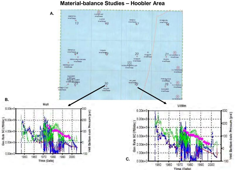
**Figure 9.6.13.** A) Map showing location of the Chase wells in the Hoobler study area. B and C) Production rate and flowingpressure history matches at Muller (Mull) and Williams (Willm) wells located in the Hoobler study area.
