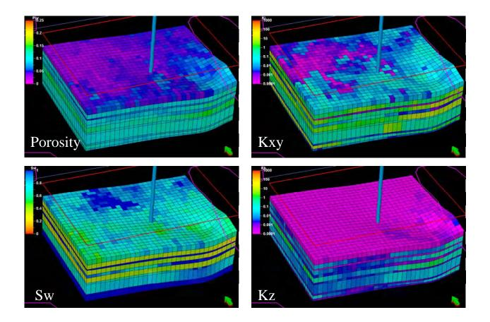
**Figure 9.5.8.** Distribution of upscaled petrophysical properties in the Hoobler 11-layer model. Hoobler well bore is shown located in the middle of the study area.
