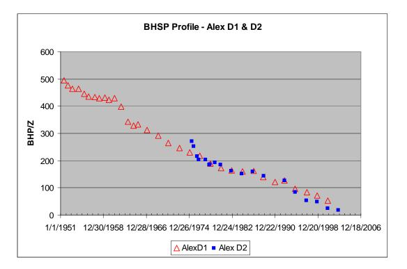
Figure 9.6.5. Plot of bottom-hole shut-in pressures recorded at Alexander D1 and D2 wells.
