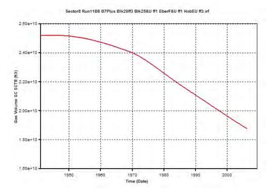
Figure 9.5.49. RUN 11 Results – Simulator-calculated gas-in-place in Fort Riley (Layer 8) through time.
