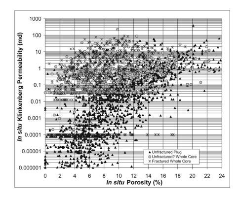
**Figure 9.3.9.** Crossplot of *in situ* Klinkenberg permeability versus *in situ* porosity for whole core identified as fractured (asterisks), whole core that were not identified as fractured but may contain microfractures (grey circle), and unfractured core plugs (black triangle).
