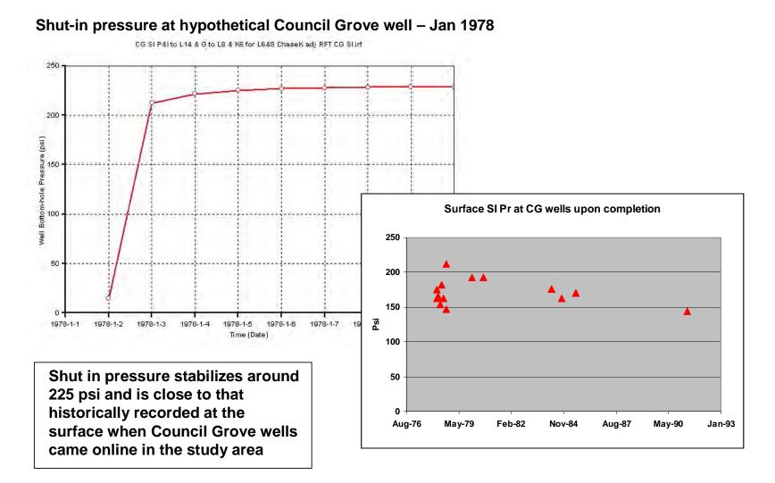
Figure 9.4.46. RUN 11 Results – Simulator-calculated shut-in pressure at a hypothetical Council Grove well as of January 1978.
