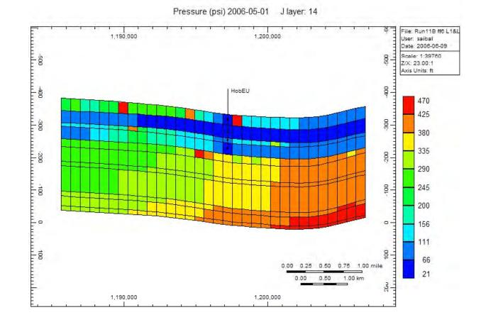
**Figure 9.5.37.** RUN 7 Results – Simulator-calculated pressure distribution along an east-west cross section through the Hoobler EU well as of May 2006.
