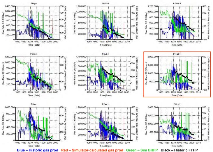
Figure 9.4.35. RUN 10 Results – Production and pressure history matches at the Chase Parent wells.
