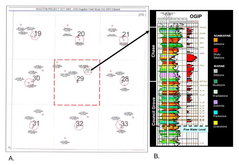
Figure 9.2.1. A) Map showing location of Alexander D1 and D2 wells. B) Well profile for the type well Alexander D2.
