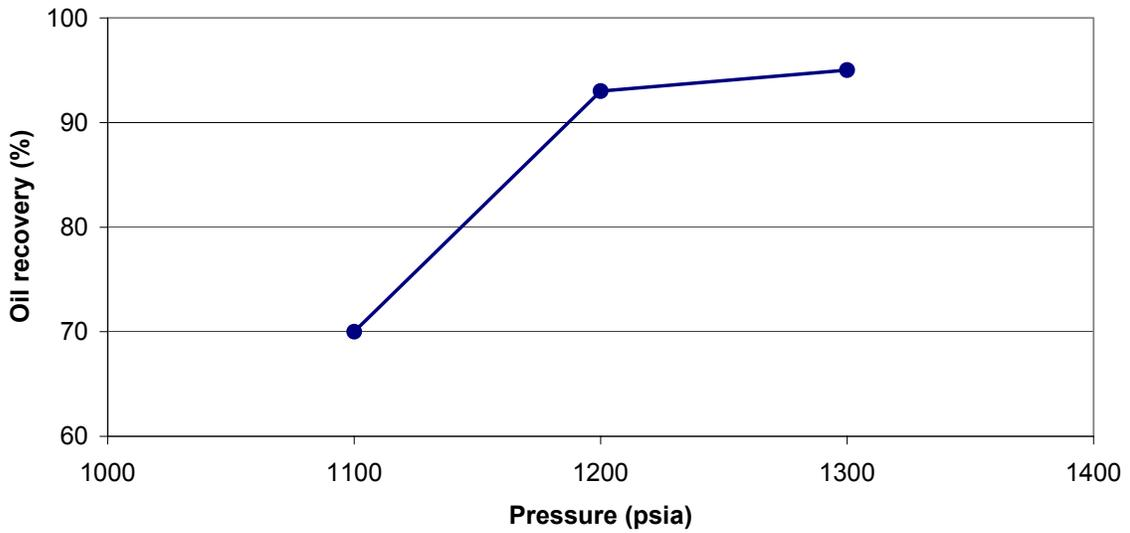
**Figure A6** - Oil recovery (at 1.2 HCPV injection of CO<sub>2</sub>) as a function of pressure for Illinois oil sample at 111 °F.
