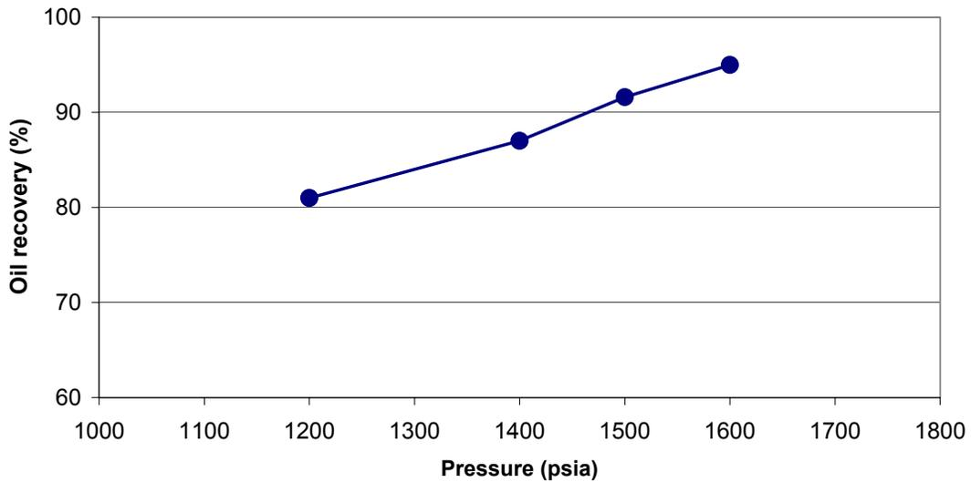
**Figure A8** - Oil recovery (at 1.2 HCPV injection of CO<sub>2</sub>) as a function of pressure for Ohio oil sample at 107 °F.
