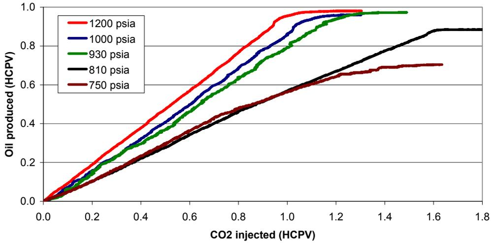
**Figure A3** - Oil recovery results in slim-tube experiment with CO<sub>2</sub> displacing Kentucky oil sample #22 at 79 °F.
