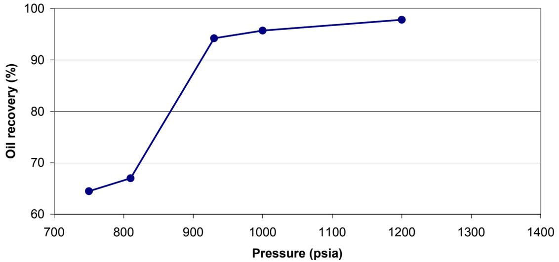
**Figure A4** - Oil recovery (at 1.2 HCPV injection of CO<sub>2</sub>) as a function of pressure for Kentucky oil sample #22 at 79 °F.
