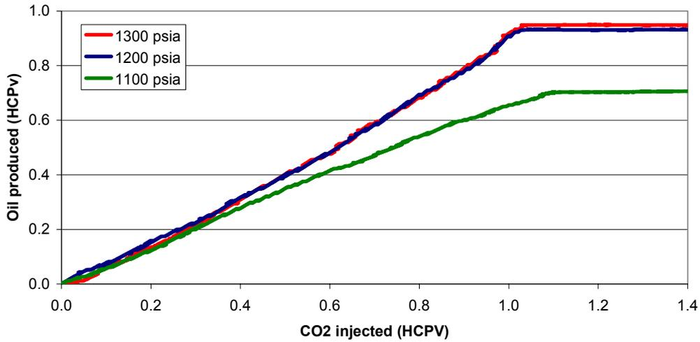
**Figure A5** - Oil recovery results in slim-tube experiment with CO<sub>2</sub> displacing Illinois oil sample at 111 °F.
