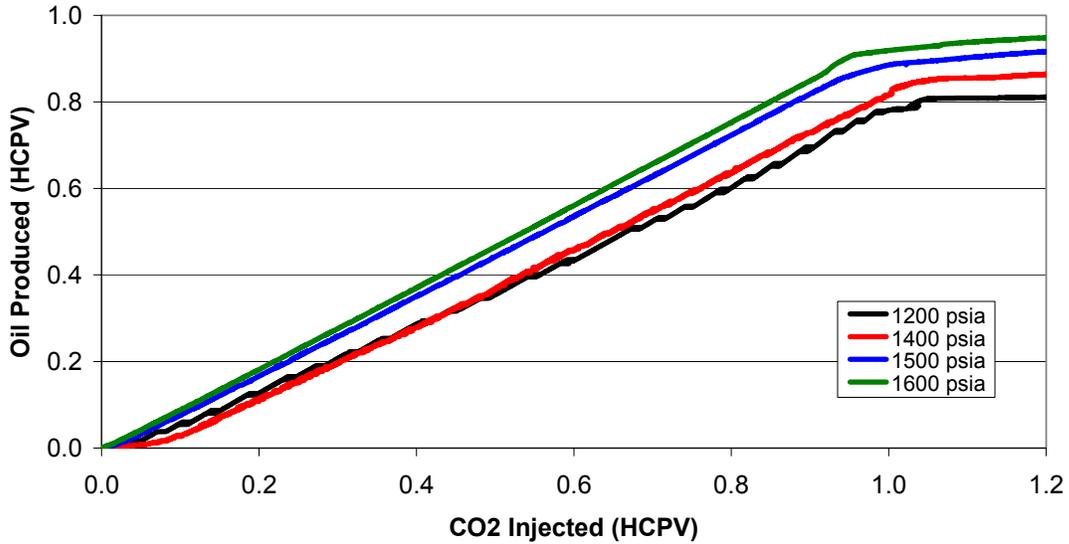
**Figure A7** - Oil recovery results in slim-tube experiment with CO<sub>2</sub> displacing Ohio oil sample at 107 °F.
