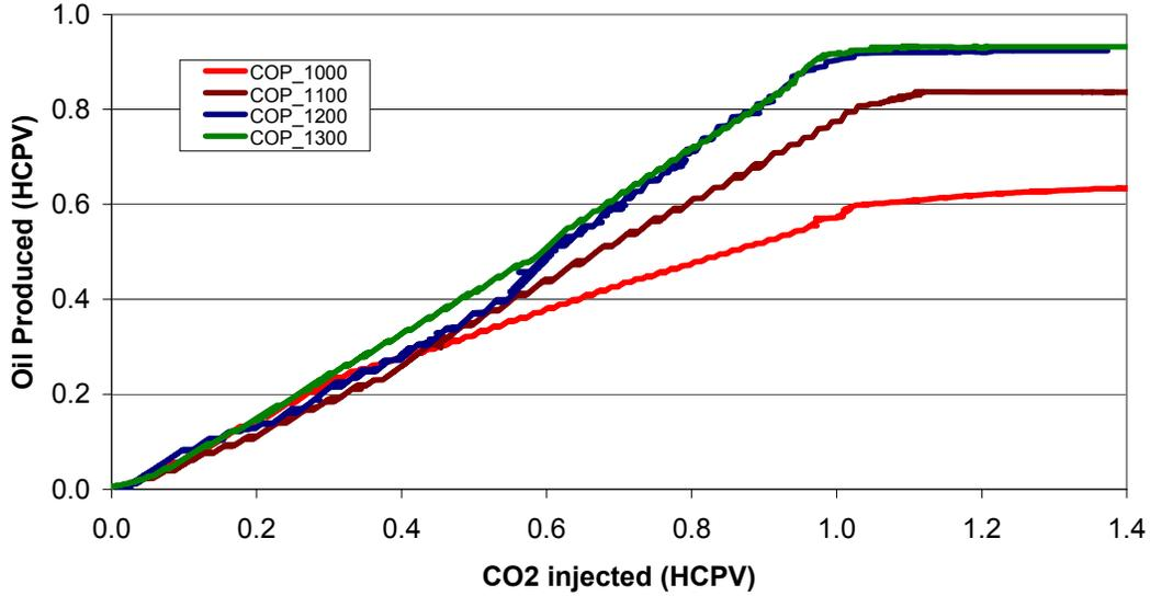
**Figure A1** - Oil recovery results in slim-tube experiment with CO<sub>2</sub> displacing Indiana oil sample at 101 °F.
